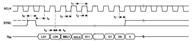
Figure 1. Serial Write Operation
