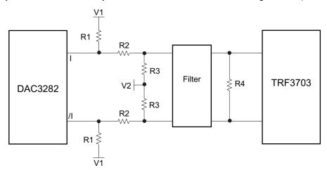
Figure 83. DAC3282 to Modulator Interface with Filter
