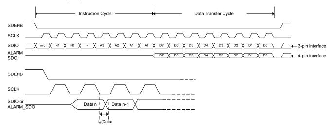
Figure 41. Serial Interface Read Timing Diagram
