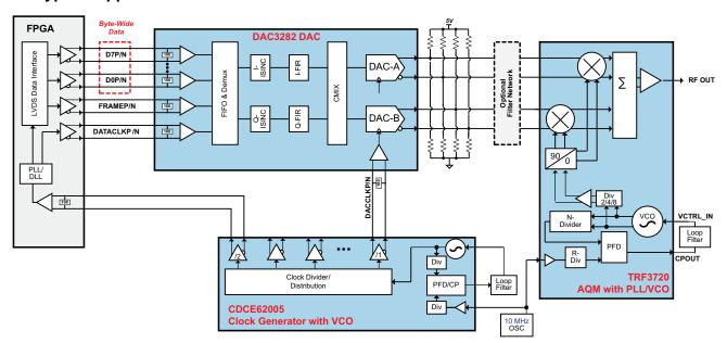
Figure 84. System Diagram of Direct Conversion Radio
