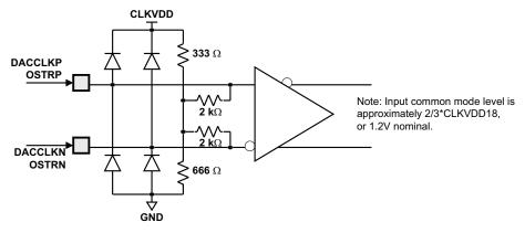
Figure 35. DACCLKP/N and OSTRP/N Equivalent Input Circuit
