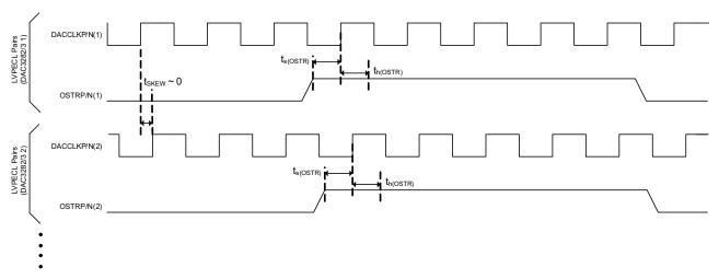
Figure 75. Timing Diagram for LVPECL Synchronization Signals
