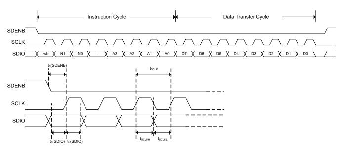
Figure 40. Serial Interface Write Timing Diagram
