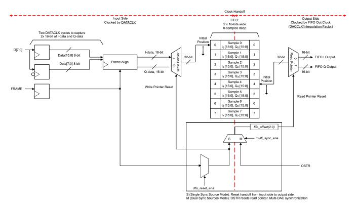
Figure 24. DAC3282 FIFO Block Diagram
