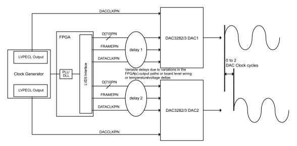
Figure 76. Multi-Device Operation in Single Sync Source Mode
