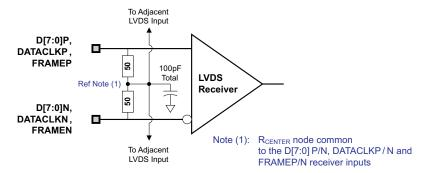
Figure 37. D[7:0]P/N, DATACLKP/N and FRAMEP/N LVDS Input Configuration
