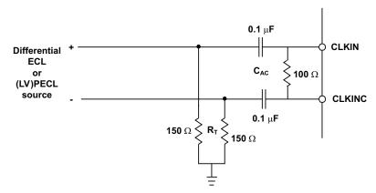
Figure 36. Preferred Clock Input Configuration With a Differential ECL/PECL Clock Source
