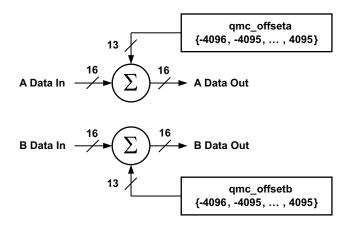
Figure 33. Digital Offset Block Diagram
