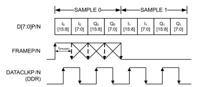
Figure 34. Byte-Wide Data Transmission Format
