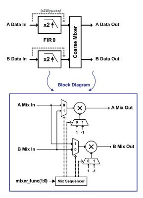
Figure 32. Coarse Mixers Block Diagram
