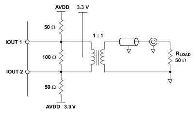
Figure 78. Driving a Doubly Terminated 50 Ω Cable Using a 1:1 Impedance Ratio Transformer
