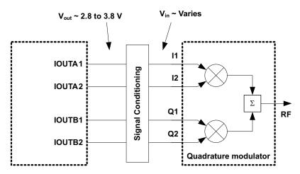
Figure 80. DAC to Analog Quadrature Modulator Interface
