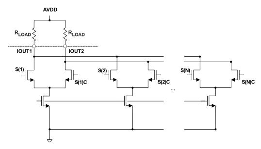
Figure 77. Equivalent Analog Current Output
