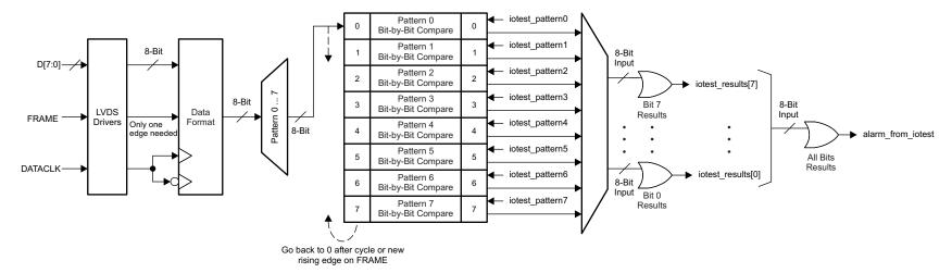
Figure 27. DAC3282 Pattern Check Block Diagram
