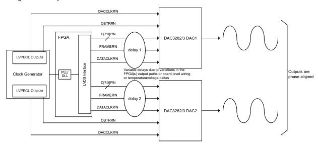
Figure 74. Synchronization System in Dual Sync Sources Mode with PLL Bypassed
