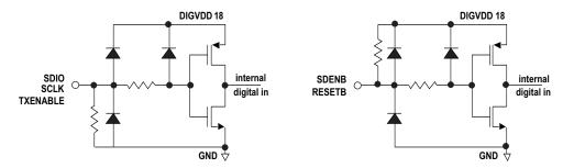
Figure 39. CMOS/TTL Digital Equivalent Input
