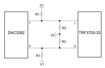
Figure 82. DAC3282 to TRF3703-33 Interface
