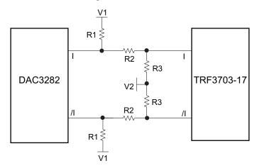
Figure 81. DAC3282 to TRF3703-17 Interface
