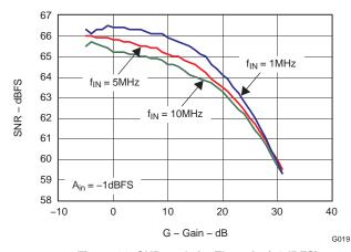
Figure 29. SNR vs Gain, Three f<sub>IN</sub> (-1dBFS)
