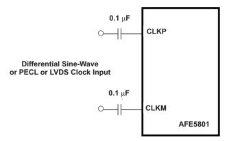
Figure 40. Differential Clock Driving Circuit
