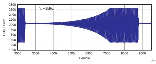
Figure 26. TGC Sweep With Interpolation Enabled and High-Pass Filter Disabled
