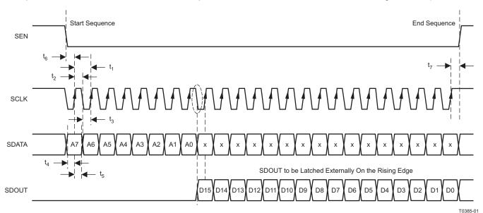
Figure 37. Serial Interface Register Read
