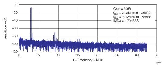
Figure 27. Intermodulation Distortion
