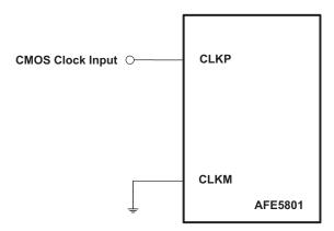
Figure 41. Single-Ended Clock Driving Circuit
