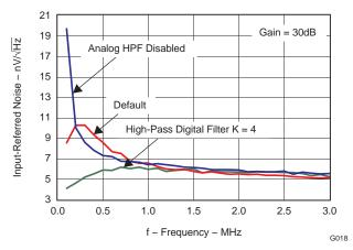
Figure 28. Input-Referred Noise vs Frequency
