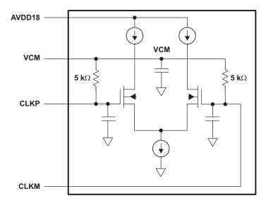
Figure 39. Internal Clock Buffer for Differential Clock Mode
