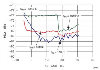
Figure 11. HD2 Across Coarse Gain and Three  $f_{IN}$  (-6dBFS)<sup>(2)</sup>
