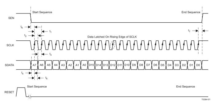
Figure 36. Serial Interface Register Write
