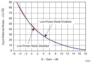
11 10 9 8 Low-Power Mode Disabled 7 6 Low-Power Mode Enabled 5 Low-Power Mode Enabled 17 18 19 20 21 22 23 24 25 26 27 28 29 30 31 G - Gain - dB
