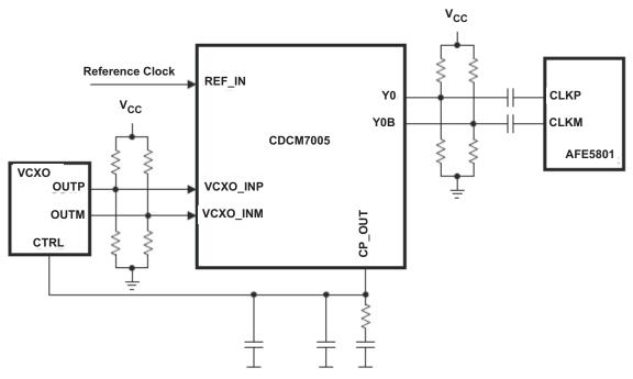
Figure 42. PECL Clock Drive Using CDCM7005
