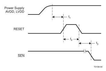
Figure 35. Reset Timing
