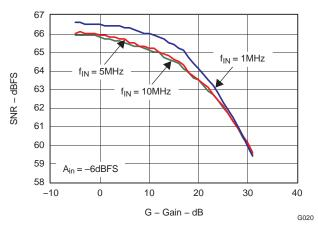
Figure 30. SNR vs Gain Three f<sub>IN</sub> (-6dBFS)
