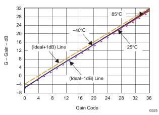
Figure 4. Fine Gain vs Gain Code
