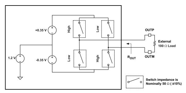
Figure 43. LVDS Output Circuit
