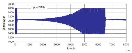
Figure 25. TGC Sweep With Interpolation Disabled and High-Pass Filter Disabled
