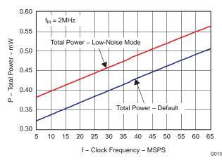
Figure 20. Analog Power vs Input-Clock Frequency
