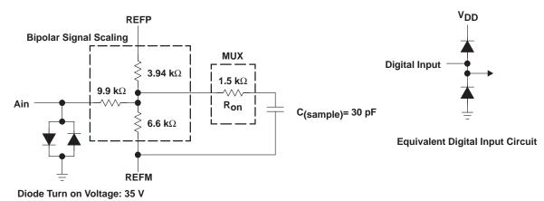
**Equivalent Analog Input Circuit**
