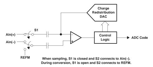
Figure 6. Simplified Pseudodifferential Input Circuit
