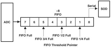
Figure 20. FIFO Structure
