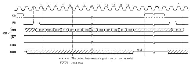
Figure 8. Write Cycle, FS Initiates Operation
