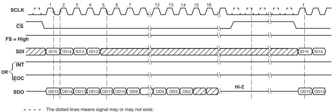
OD[15:2] (for TLC3574/78) or OD[15:4](for TLC2574/78) is the FIFO content.
