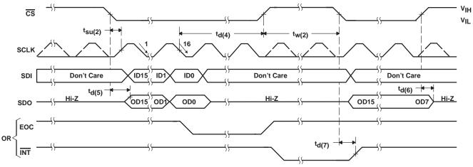
The dotted line means signal may or may not exist, depending on application. It must be ignored. Normal sampling mode, CS initiates the conversion, FS must be tied to high. When CS is high, SDO is in Hi-Z, all inputs (FS, SCLK, SDI) are inactive and are ignored.
