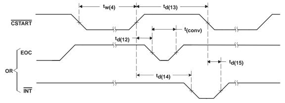
Figure 4. Critical Timing for Extended Sampling (CSTART Trigger)
