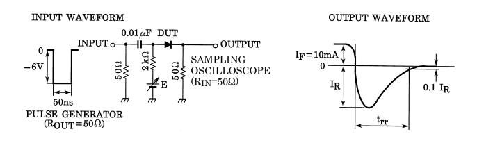
Fig.1 Reverse Recovery Time (trr) Test Circuit
