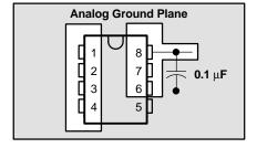
Figure 16. Power-Supply Bypassing
