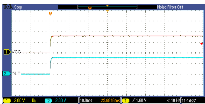
Figure 15. TMP303A Power-On Response, T_A Greater Than 60°C
