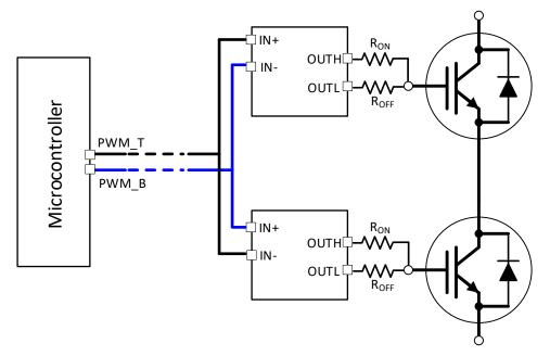
Figure 9-2. PWM Interlock for a Half Bridge
