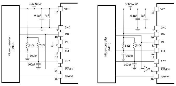
Figure 9-4. Automatic Reset Control
