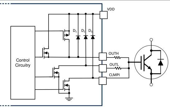
Figure 8-3. Short Circuit Clamping
