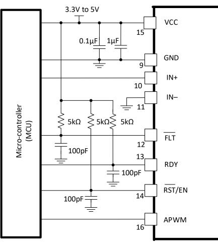
Figure 9-3. FLT, RDY and RST/EN Pins Circuitry
