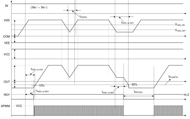
Figure 7-9. VDD UVLO Protection Timing Diagram
