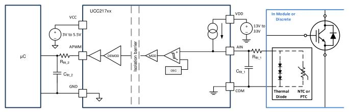
Figure 9-11. APWM Channel with Filtered Output
