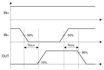
Figure 7-2. Inverting Logic Propagation Delay Measurement
