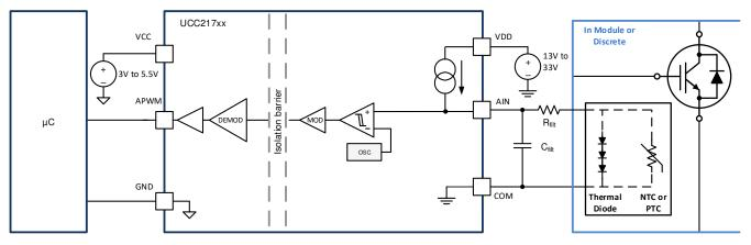
Figure 9-10. Thermal Diode or Thermistor Temperature Sensing Configuration
