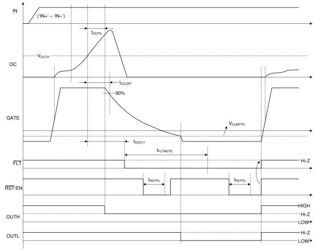
Figure 7-10. OC Protection with Soft Turn-OFF
