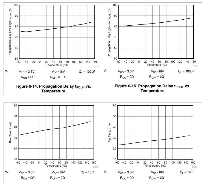
Figure 6-16. t<sub>r</sub> Rise Time vs. Temperature
