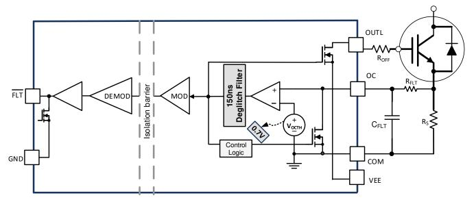
Figure 8-5. Overcurrent and Short Circuit Protection
