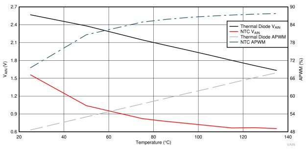
Figure 9-12. Thermal diode and NTC V<sub>AIN</sub> and Corresponding Duty Cycle at APWM
