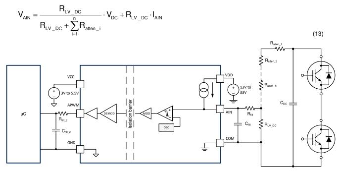
Figure 9-15. DC-link Voltage Sensing Configuration
