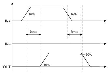
Figure 7-1. Non-inverting Logic Propagation Delay Measurement
