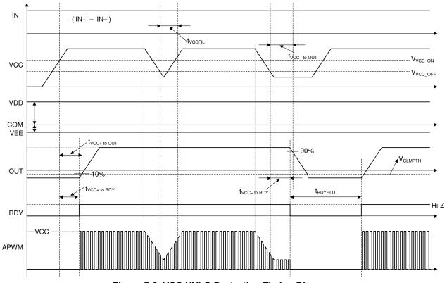
Figure 7-8. VCC UVLO Protection Timing Diagram
