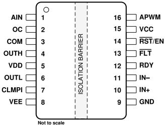
Figure 5-1. UCC21710 DW SOIC (16) Top View
