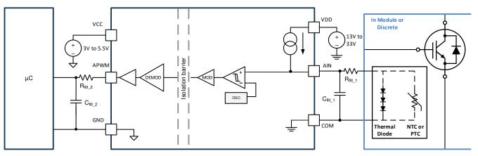
Figure 8-7. Isolated Analog to PWM Signal
