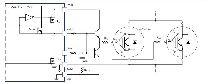
Figure 9-16. Current Buffer for Increased Drive Strength
