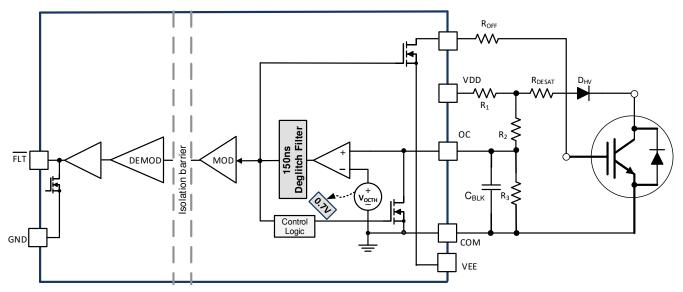
Figure 9-8. Overcurrent and Short Circuit Protection Based on Desaturation Circuit
