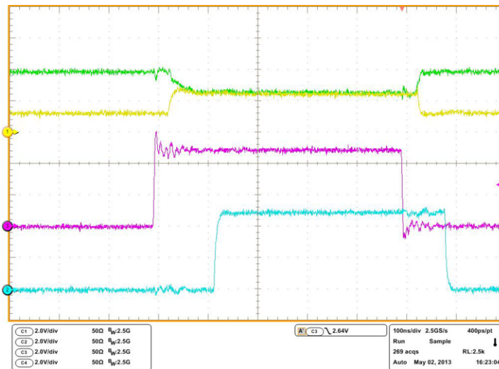
Figure 21. Typical TXD to RXD Loop Delay
