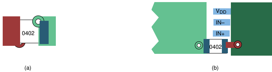
图 11-7. Typical Decoupling Capacitor Layouts
