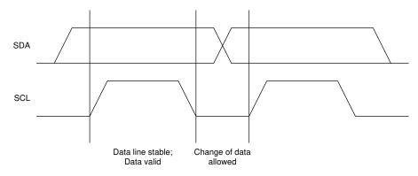
图 8-7. Bit Transfer on the I<sup>2</sup>C Bus
