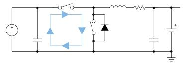
图 11-1. High Frequency Current Path
