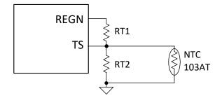
图 8-5. TS Pin Resistor Network
