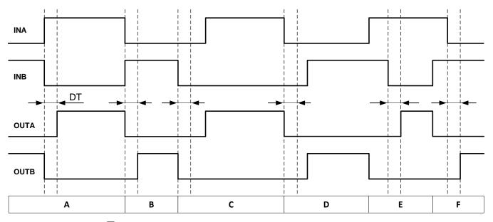
图 35. Input and Output Logic Relationship with Input Signals
