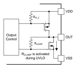
图 32. Simplified Representation of Active Pull Down Feature
