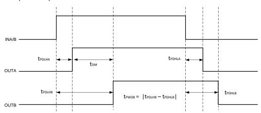
图 25. Delay Matching and Pulse Width Distortion
