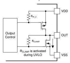
Figure 9-1. Simplified Representation of Active Pull Down Feature
