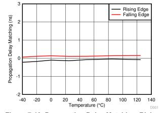
Figure 7-19. Propagation Delay Matching, Rising and Falling Edge
