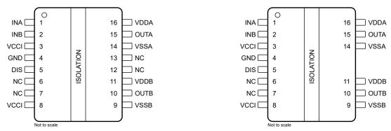
Figure 6-3. DW Package 16-Pin SOIC Top View
