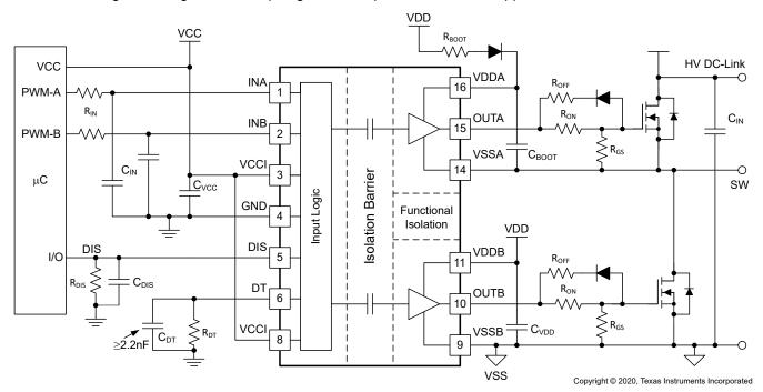
Figure 10-1. Typical Application Schematic
