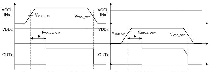
Figure 8-7. VCCI Power-up UVLO Delay
