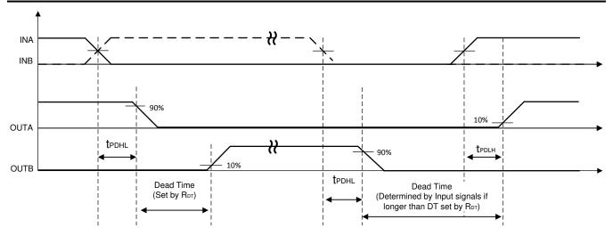
Figure 8-6. Dead Time Switching Parameters for UCC21540/A, UCC21541
