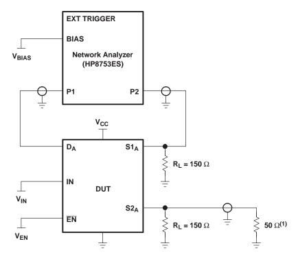
(1) A 50- $\Omega$  termination resistor is needed for the network analyzer.
