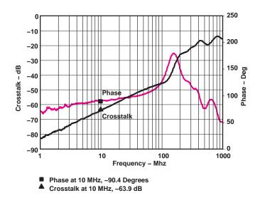
Figure 4. Crosstalk vs Frequency
