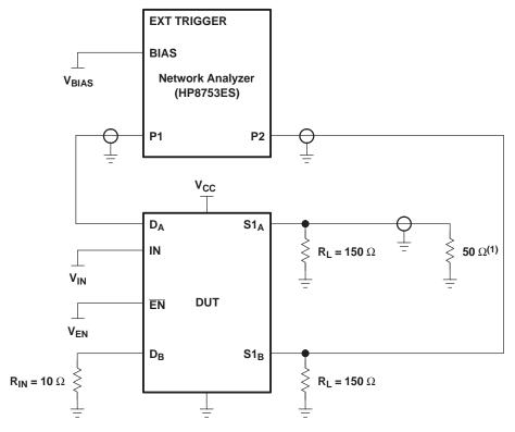
(1) A 50- $\Omega$  termination resistor is needed for the network analyzer.
