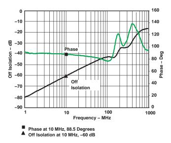
Figure 3. Off Isolation vs Frequency
