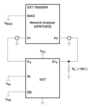
Figure 7. Test Circuit for Frequency Response (BW)
