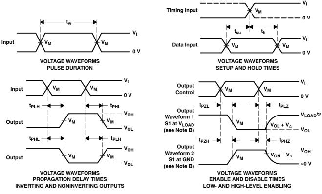
NOTES: A. CL includes probe and jig capacitance.
