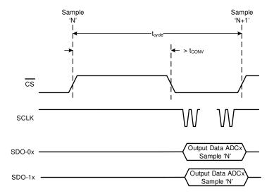
图 6-1. Conversion Control Latency-0 Data Capture
