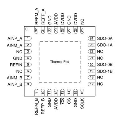
图 5-1. RHB Package, 5-mm × 5-mm, 32-Pin VQFN, Top View
