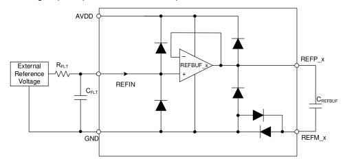
图 7-4. Connection Diagram for Reference and Reference Buffers
