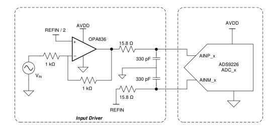
图 8-2. Typical Connection Diagram of the ADS9226 Application Circuit
