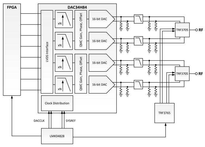
Figure 93. Zero LTE Transmitter Diagram
