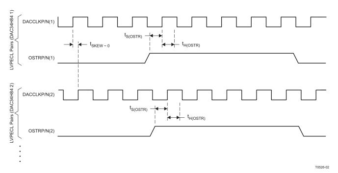
Figure 85. Timing Diagram for LVPECL Synchronization Signals
