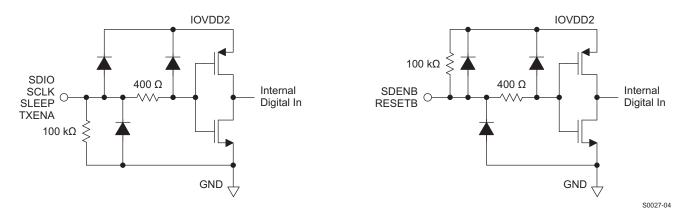
Figure 81. CMOS Digital Equivalent Input
