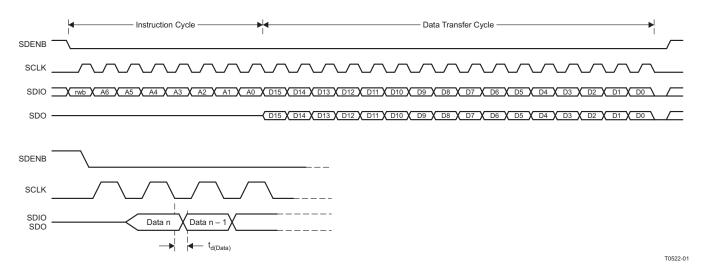
Figure 50. Serial Interface Read Timing Diagram
