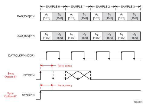
Figure 51. Data Transmission Format
