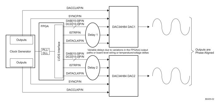
Figure 86. Synchronization System in Dual Sync Sources Mode with PLL Enabled
