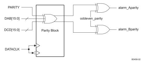
Figure 75. DAC34H84 32-Bit Parity Check
