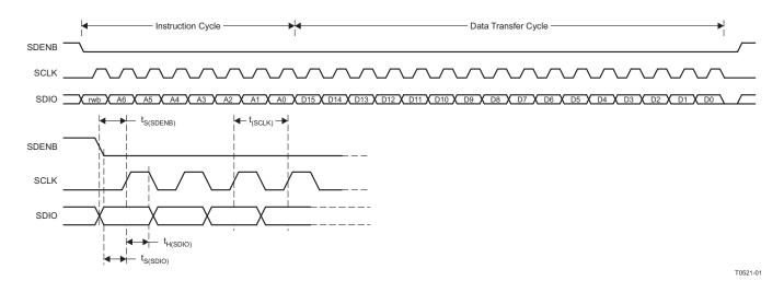
Figure 49. Serial Interface Write Timing Diagram
