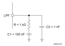
Figure 57. Recommended External Loop Filter
