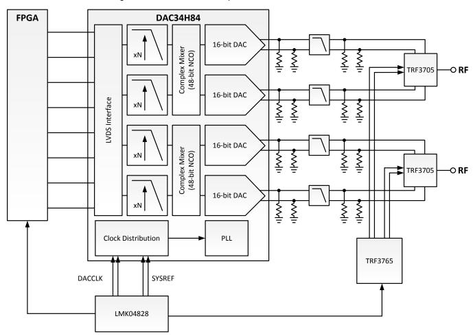
Figure 88. Dual Low-IF Wideband LTE Transmitter Diagram
