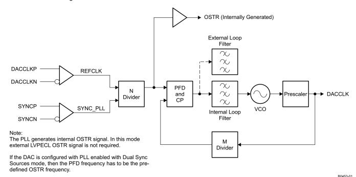
Figure 55. PLL Block Diagram
