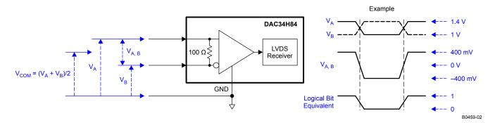
Figure 80. LVDS Data Input Levels
