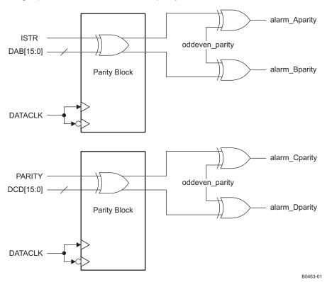
Figure 76. DAC34H84 Dual 16-Bit Parity Check
