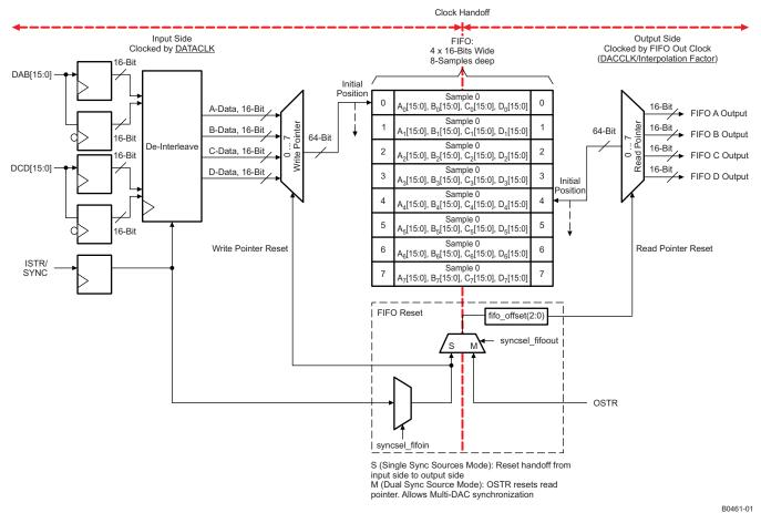
Figure 52. DAC34H84 FIFO Block Diagram
