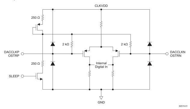
Figure 77. DACCLKP/N and OSTRP/N Equivalent Input Circuit
