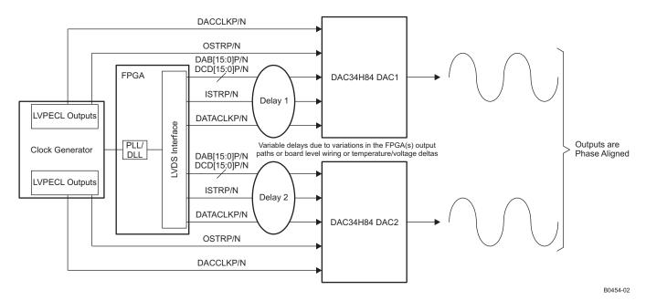
Figure 84. Synchronization System in Dual Sync Sources Mode with PLL Bypassed
