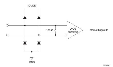
Figure 79. DAB[15:0]P/N, DCD[15:0]P/N, DATACLKP/N, ISTRP/N, SYNCP/N and PARITYP/N LVDS Input Configuration
