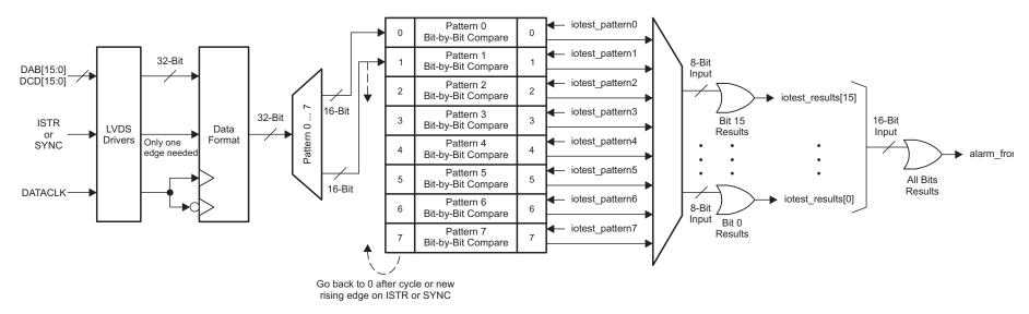
Figure 74. DAC34H84 Pattern Check Block Diagram
