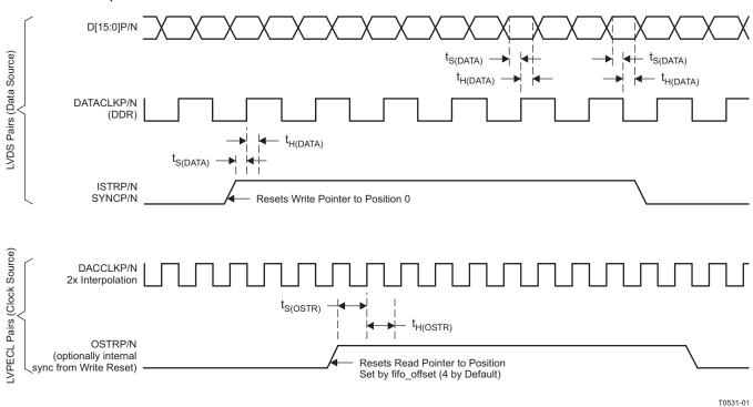
Figure 53. FIFO Write and Read Descriptions
