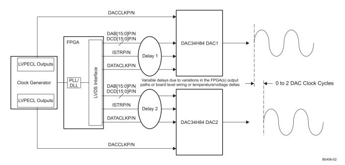
Figure 87. Multi-Device Operation in Single Sync Source Mode
