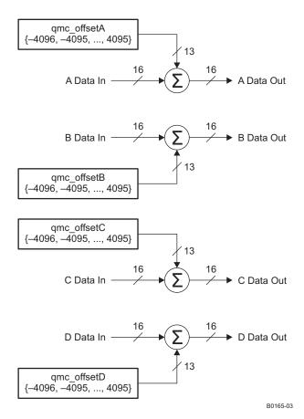
Figure 72. Digital Offset Block Diagram
