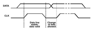
Figure 33. Bit Transfer on the Serial Interface
