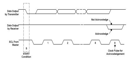
Figure 34. Acknowledge on the I<sup>2</sup>C Bus
