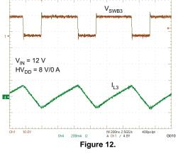
BUCK 3 (HV<sub>DD</sub>) PWM SWITCHING – HEAVY LOAD
