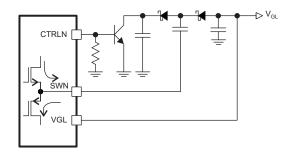
Figure 28. Negative Charge Pump Application Circuit
