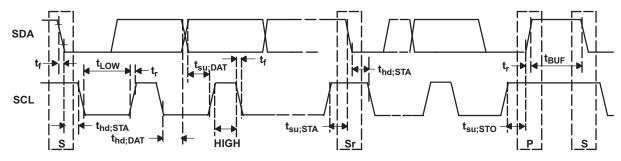
Figure 1. Serial Interface Timing for F/S-Mode
