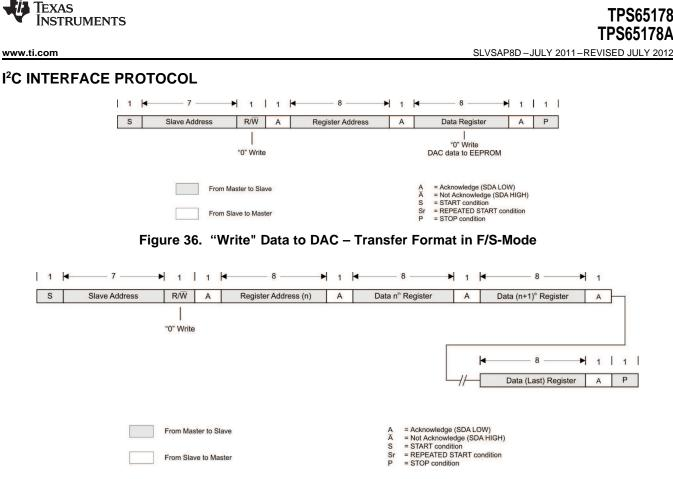
Figure 37. "Write" Data to DAC - Transfer Format in F/S-Mode Featuring Register Address Auto-Increment
