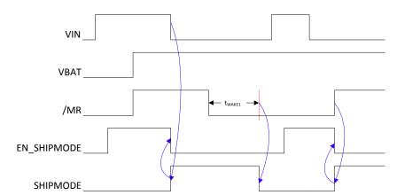
图 28. Ship Mode Entry Based On EN\_SHIPMODE bit
