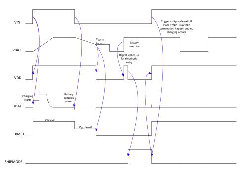
图 29. BQ21061 Wake-Up Upon Supply Insertion
