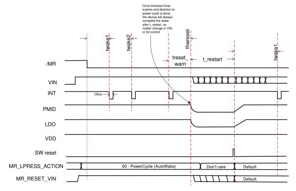
图 20. MR Wake and Reset Timing with VIN Present or BAT Active Mode When MR\_LPRESS\_ACTION =
