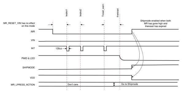
图 21. MR Wake and Reset Timing Active Mode When MR\_LPRESS\_ACTION = 1x (Ship Mode) and Only **BAT** is Present
