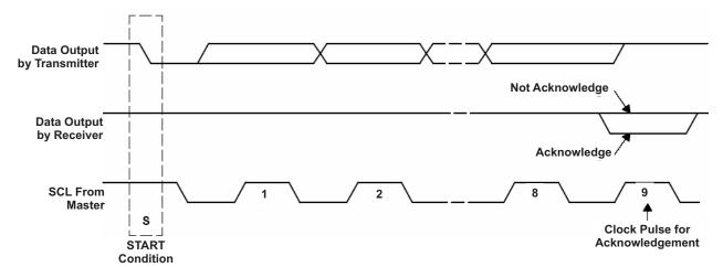
图 26. Acknowledge on the I<sup>2</sup>C Bus
