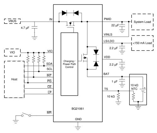
图 61. Typical Application Diagram
