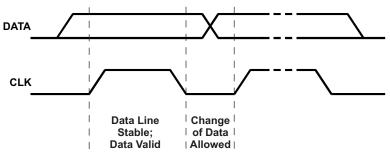
图 25. Bit Transfer on the Serial Interface
