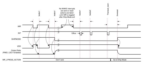
图 18. MR Wake from Ship Mode (MR\_LPRESS\_ACTION = Ship Mode, VIN not valid)
