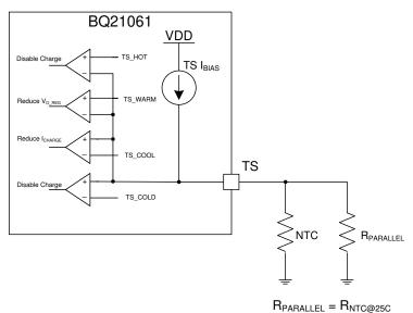
图 23. TS Bias Functional Diagram
