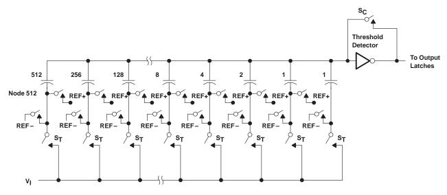
Figure 1. Simplified Model of the Successive-Approximation System
