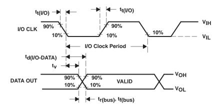
Figure 11. DATA OUT and I/O CLK Voltage Waveforms
