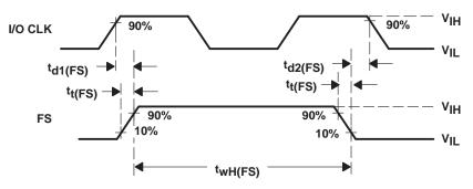
Figure 14. FS and I/O CLK Voltage Waveforms
