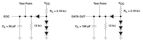
Figure 7. Load Circuits
