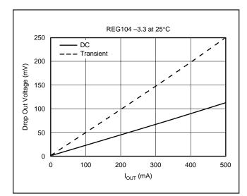
FIGURE 8. Transient and DC Dropout.
