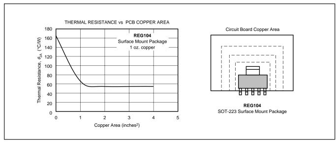
FIGURE 11. Thermal Resistance versus PCB Area for the Five Lead SOT-223.
