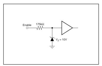
FIGURE 3. Enable Pin Equivalent Input Circuit.
