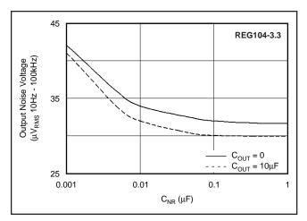
FIGURE 6. Output Noise versus Noise Reduction Capacitor.
