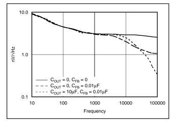
FIGURE 7. Output Noise Density on Adjustable Versions.
