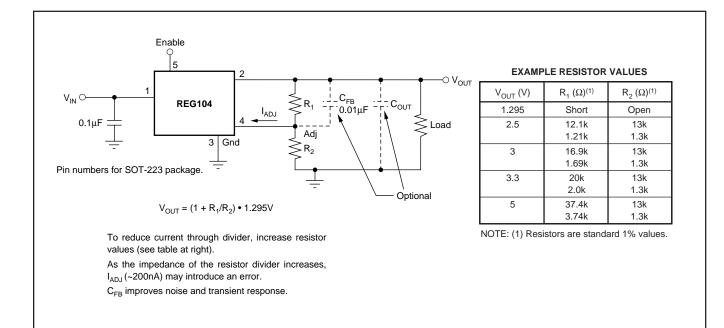
FIGURE 2. Adjustable Voltage Circuit for REG104A.
