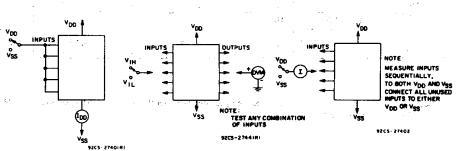
Fig. 9 — Quiescent device current test circuit.
