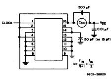
Fig.17 – Dynamic power dissipation test circuit (÷ 2 mode).
