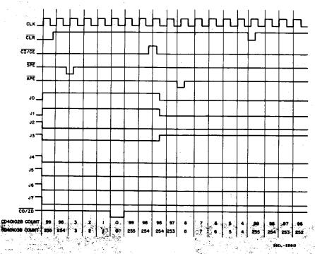
Fig. 15 - Timing diagram for CD40102B and CD40103B.
