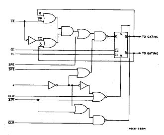
Fig. 14 — Detail logic diagram for flip-flops, FFO — FF7, used in logic diagrams for CD401028 and CD40103B.
