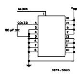
Fig.16 - Maximum clock frequency test circuit.
