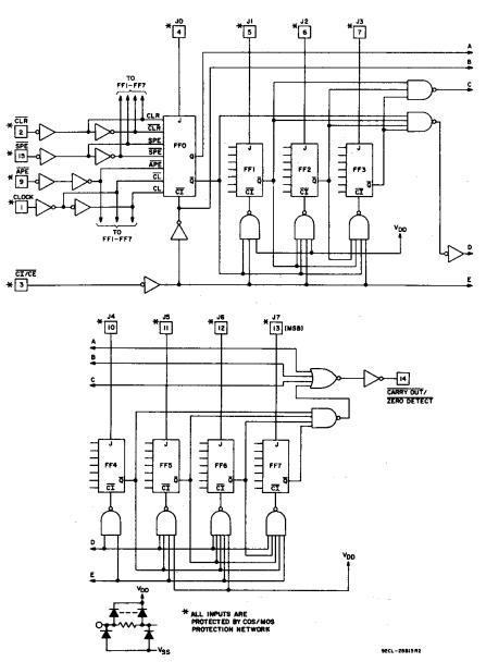
Fig. 13 — Logic diagram for CD40103B.
