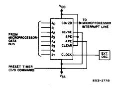
Fig.20 - Microprocessor interrupt timer.
