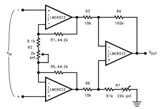
$\begin{array}{l} \text{If R1} = \text{R5, R3} = \text{R6, and R4} = \text{R7;} \\ \frac{\text{V}_{\text{OUT}}}{\text{V}_{\text{IN}}} = \frac{\text{R2} + 2\text{R1}}{\text{R2}} \times \frac{\text{R4}}{\text{R3}} \end{array}$
