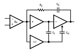
Figure 2. LMC6022 Circuit Topology (Each Amplifier)
