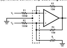
Figure 30. Guard Ring Connections
