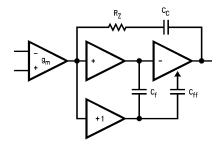
Figure 26. LMC6022 Circuit Topology (Each Amplifier)
