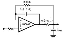
Figure 27. Rx, Cx Improve Capacitive Load Tolerance
