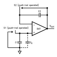
Figure 32. Simple Input Bias Current Test Circuit
