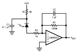
**Note:** A 5V bias on the photodiode can cut its capacitance by a factor of 2 or 3, leading to improved response and lower noise. However, this bias on the photodiode will cause photodiode leakage (also known as its dark current).
