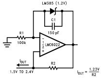
(Upper limit of output range dictated by input common-mode range; lower limit dictated by minimum current requirement of LM385.)
