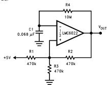
Figure 38. 1 Hz Square-Wave Oscillator
