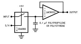
Figure 35. Low-Leakage Sample-and-Hold
