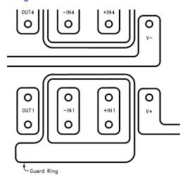
Figure 29. Example of Guard Ring in P.C. Board Layout (Using the LMC6024)
