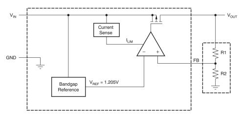
Figure 1. Adjustable Voltage Version
