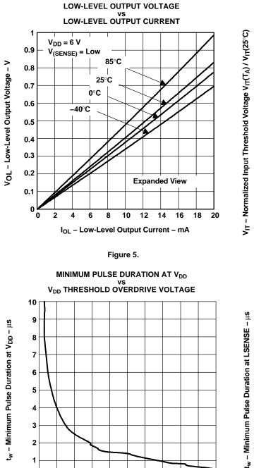
9  $t_w$  – Minimum Pulse Duration at V<sub>DD</sub> –  $\mu$ s 8 7 6 5 4 3 2 1 0 0.1 0.2 0.3 0.4 0.5 0.6 0.7 0.8 0.9 0 1 V<sub>DD</sub> – Threshold Overdrive Voltage – V Figure 7.
