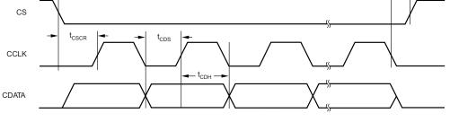
Figure 64. SPI Port Timing
