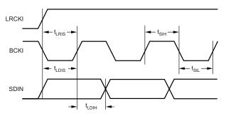
Figure 60. Input Port Timing
