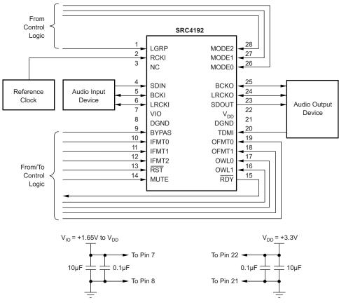
Figure 76. Typical Connection Diagram for the SRC4192
