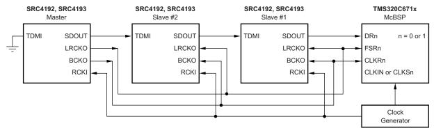
Figure 75. TDM Interface where one Device is Master to Multiple Slaves
