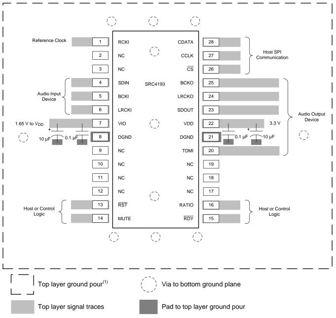
(1) TI recommends placing a top-layer ground pour for shielding around the SRC4193 device and connecting it to the lower main PCB-ground plane with multiple vias.
