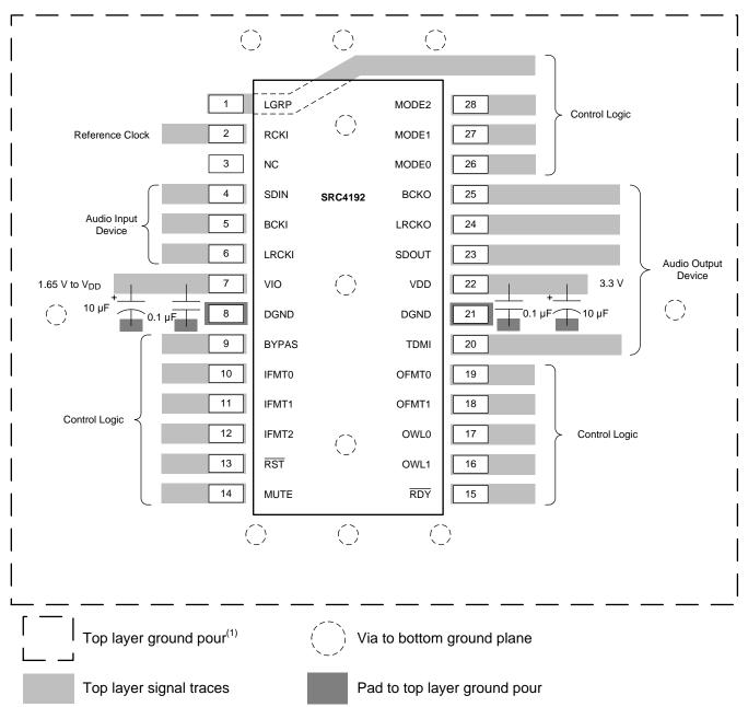
(1) TI recommends placing a top-layer ground pour for shielding around the SRC4192 device and connecting it to the lower main PCB-ground plane with multiple vias.
