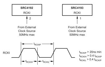
Figure 80. Reference Clock Input Connections and Timing Requirements
