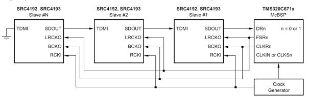
Figure 74. TDM Interface where all Devices are Slaves
