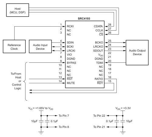
Figure 77. Typical Connection Diagram for the SRC4193
