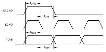
Figure 73. Input Timing for TDM Mode
