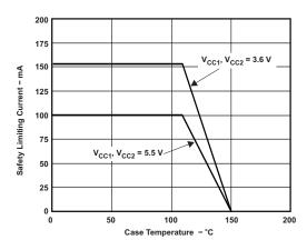
Figure 8.  $\theta_{JC}$  Thermal Derating Curve Per IEC 60747-5-2
