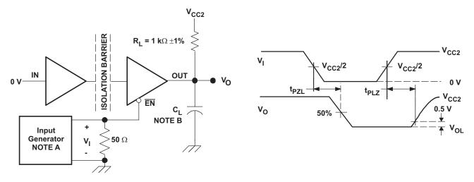
Figure 3. ISO722-Q1 Sleep-Mode Low-Level Output Test Circuit and Voltage Waveforms
