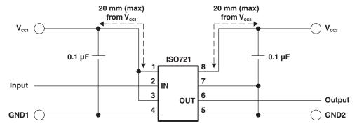
Figure 18. Basic Application Circuit
