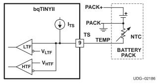
Figure 6. Temperature Sensing Configuration
