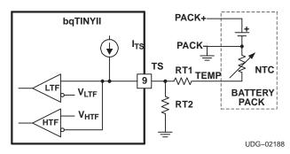
Figure 7. Temperature Sensing Thresholds
