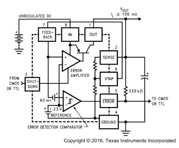
Figure 16. LP2954 SOIC Functional Block Diagram
