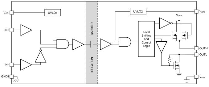
图 49. Functional Block Diagram — Split Output (UCC53x0S)
