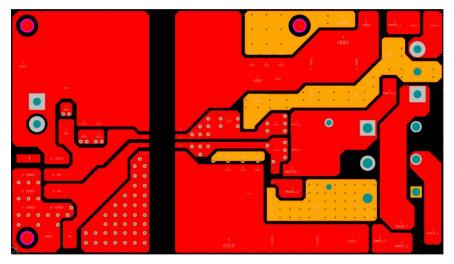
图 64. Top-Layer Traces and Copper
