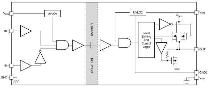
图 51. Functional Block Diagram — UVLO With Respect to GND2 (UCC53x0E)
