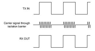
图 48. On-Off Keying (OOK) Based Modulation Scheme
