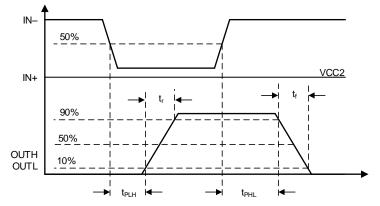
图 43. OUTH and OUTL Propagation Delay, Inverting Configuration
