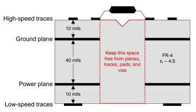
图 67. Recommended Layer Stack
