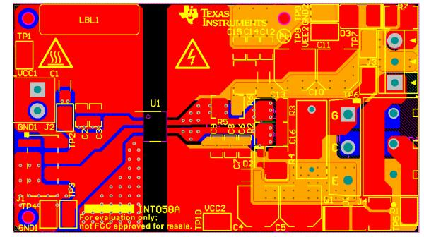
图 63 shows a PCB layout example with the signals and key components labeled.
