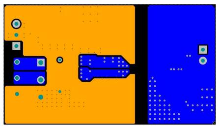
图 65. Bottom-Layer Traces and Copper (Flipped)
