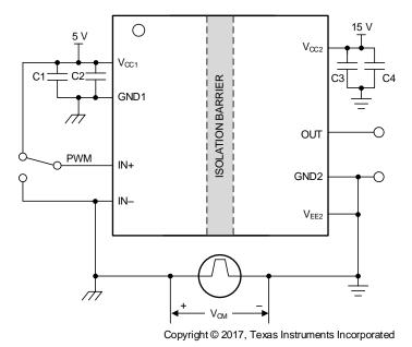
图 46. CMTI Test Circuit for UVLO2 with Respect to GND2 (UCC53x0E)
