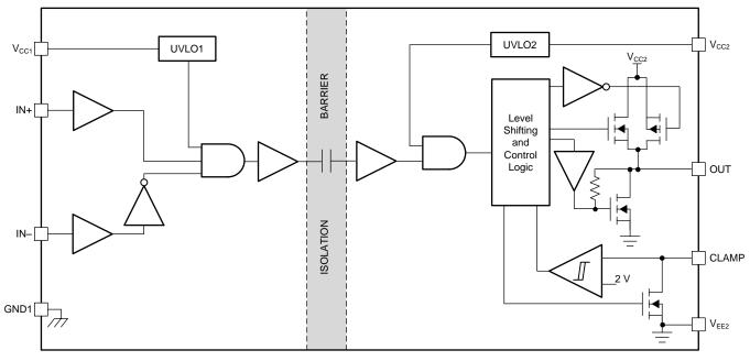
图 50. Functional Block Diagram — Miller Clamp (UCC53x0M)
