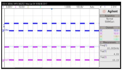
$V_{CC2} = 20 V$   $V_{EE2} = GND f_{SW} = 10 \text{ kHz}$ **2** 62. PWM Input And Gate Voltage Waveform
