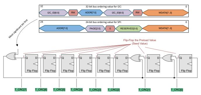
图 8-52. Calculation of 8-Bit CRC on Transmitted Data (T\_CRC)
