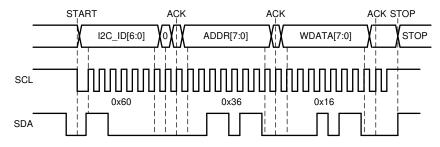
图 8-57. I<sup>2</sup>C Write Cycle without CRC
