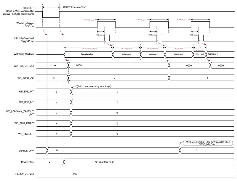
图 8-19. Watchdog in Trigger Mode - Normal MCU Start-up with Correct Watchdog-Triggers
