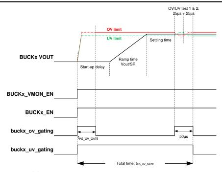
图 8-13. Timing of BUCK Regulator UV/OV Self Test
