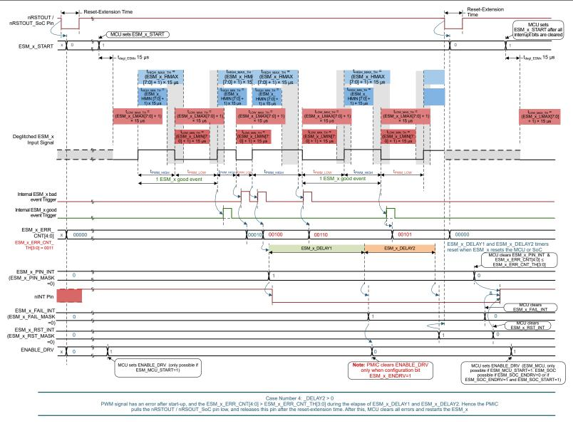
图 8-38. Example Waveform for ESM in PWM Mode - Case Number 4: ESM Starts with Low-Level at Deglitched Input Signal and Receives a Correct PWM Signal. Afterwards the ESM Detects Bad Events, and the PWM Signal Recovers Too Late which Leads to an ESM\_x Reset Trigger to the PFSM (The \_x stand for \_MCU or \_SoC)
