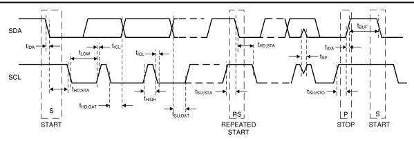
图 8-55. I<sup>2</sup>C-Compatible Timing
