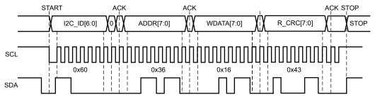
The I<sup>2</sup>C controller device (i.e. the MCU) provides R\_CRC[7:0], which is calculated from the I2C\_ID, R/W, ADDR, and the WDATA bits (24 bits). See CRC Calculation for I2C and SPI Interface Protocols.
