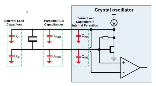
图 9-2. Crystal Oscillator Component Selection
