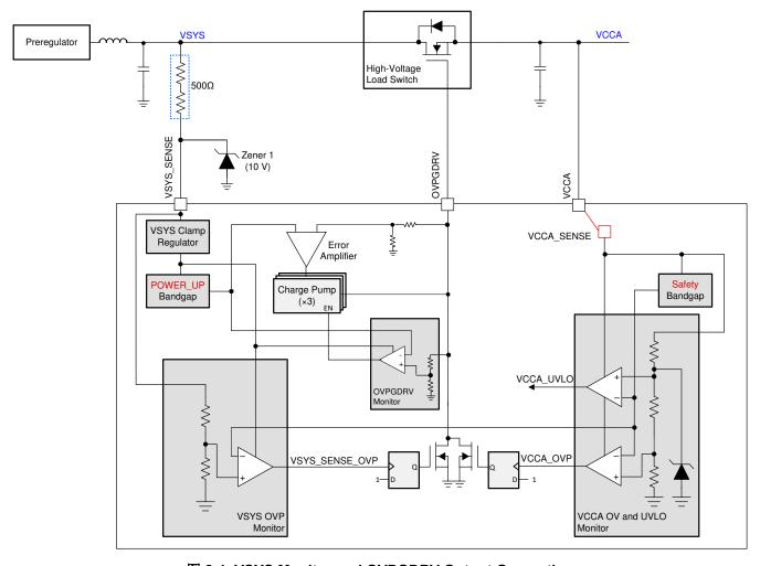
图 8-1. VSYS Monitor and OVPGDRV Output Generation
