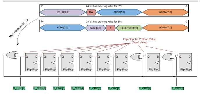
图 8-51. Calculation of 8-Bit CRC on Received Data (R\_CRC)
