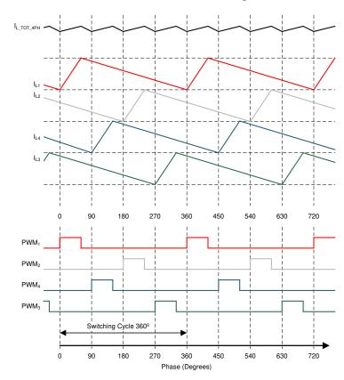
图 8-3. Example of PWM Timings, Inductor Current Waveforms, and Total Output Current in 4-Phase Configuration. <sup>1</sup>
