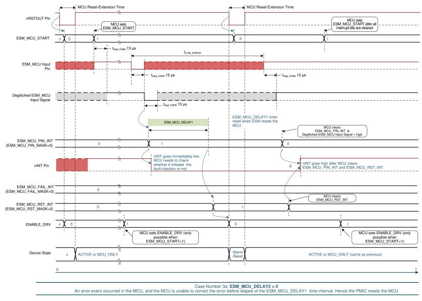
图 8-31. Example Waveform for ESM in Level Mode - Case Number 3a: Delay-2 Set To 0 and ESM\_MCU\_ENDRV=1, ESM\_MCU Input Signal Recovers Too Late and MCU-Reset Occurs
