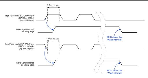
图 8-43. CAN Wake-Up Timing Diagram
