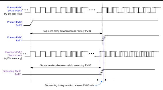
图 8-48. Multi-PMIC Rail Sequencing Timing Variation
