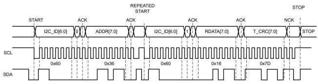
The  $I^2C$  target device (i.e. the TPS6594-Q1) provides T\_CRC[7:0], which is calculated from the  $I^2C$ \_ID, R/W, ADDR,  $I^2C$ \_ID, R/W, and the RDATA bits (32 bits). See CRC Calculation for I2C and SPI Interface Protocols.
