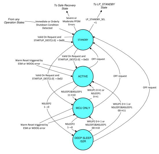
图 8-42. Example of a Mission State-Machine
