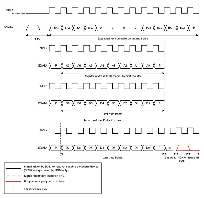
图 8-49. SPMI Extended Register Write Command
