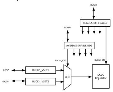
图 8-5. AVS/DVS Configuration Register Arbitration Diagram
