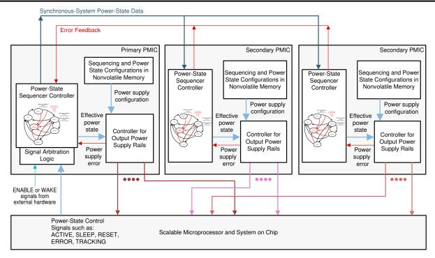
图 8-46. Multi-PMIC Power State Synchronization Block Diagram
