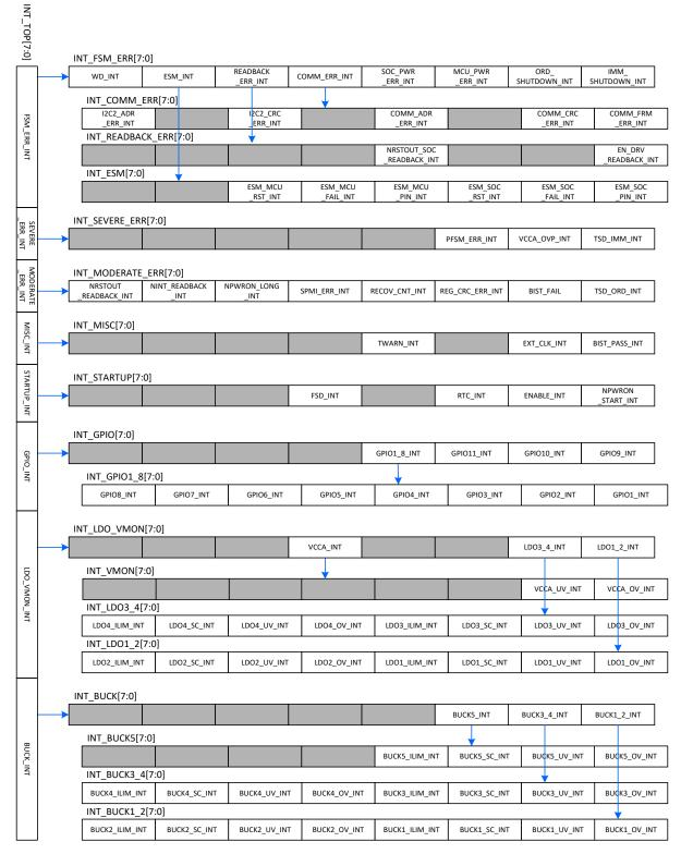
图 8-15. Hierarchical Structure of Interrupt Registers
