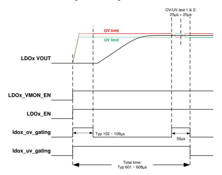
图 8-14. Timing of LDO Regulator UV/OV Self-Test
