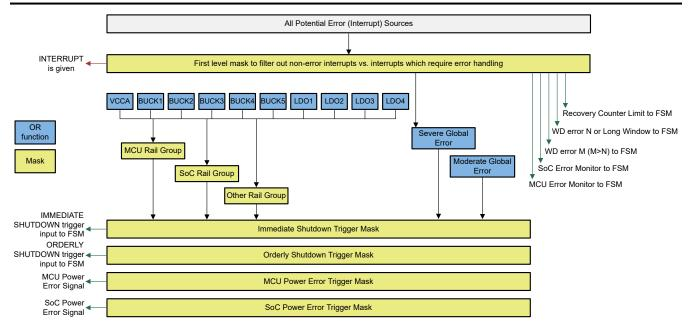
图 8-40. Error Source Hierarchical Mask System
