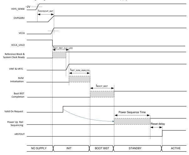
图 8-44. Device Start-up Timing Diagram
