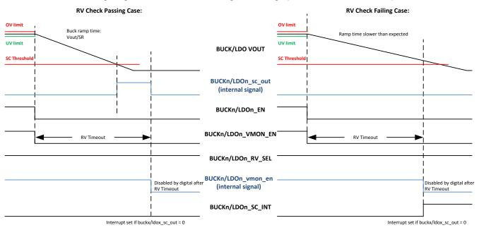
图 8-10. Residual Voltage Check Timing Diagram
