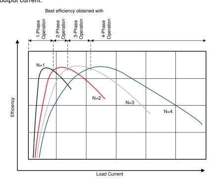
图 8-4. Multiphase BUCK Converter Efficiency vs Number of Phases (Converters in PWM Mode) <sup>2</sup>
