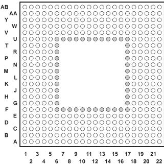
The C6203B and C6202 GLS BGA packages are pin-compatible with the C6204 GLW package except that the inner row of balls (which are additional power and ground pins) are removed for the C6204 GLW package.
