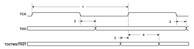
Figure 59. JTAG Test-Port Timing
