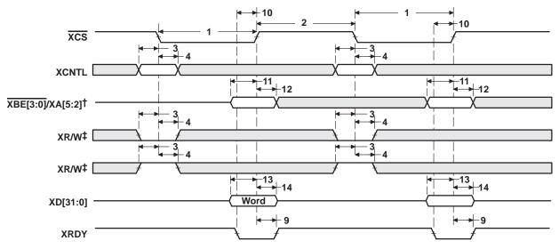
TXBE[3:0]/XA[5:2] operate as byte-enables  $\overline{XBE[3:0]}$  during host-port accesses.
