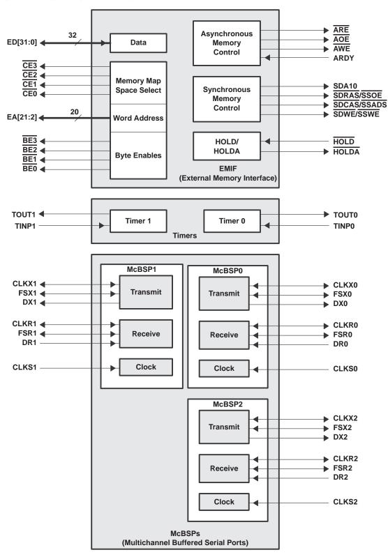
**Figure 3. Peripheral Signals**
