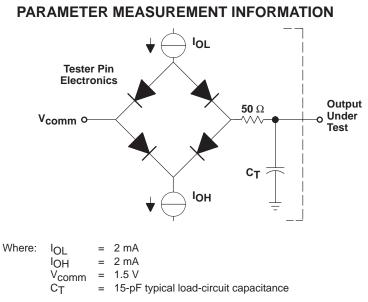
Figure 11. Test Load Circuit for AC Timing Measurements
