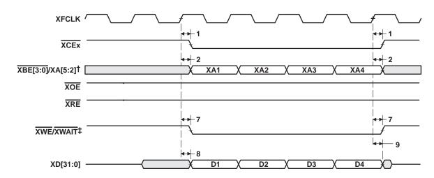
TBE[3:0]/XA[5:2] operate as address signals XA[5:2] during synchronous FIFO accesses.
