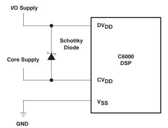
Figure 10. Schottky Diode Diagram
