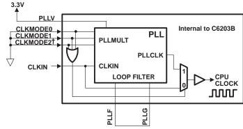
† The CLKMODE2 pin is not available for the C6203B GNZ package.
