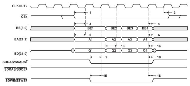
† SDCAS/SSADS, SDRAS/SSOE, and SDWE/SSWE operate as SSADS, SSOE, and SSWE, respectively, during SBSRAM accesses.
