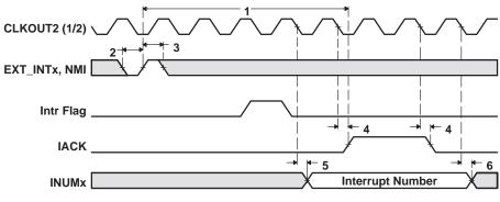
Figure 33. Interrupt Timing
