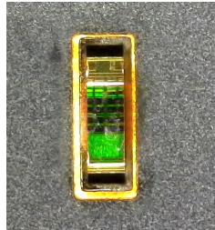
图 9-5. Image of FPCB With OPT4001 Mounted, Receiving Light Through the Cutout with a Rectangular Shape
