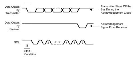
Figure 13. Bus Acknowledge Cycle
