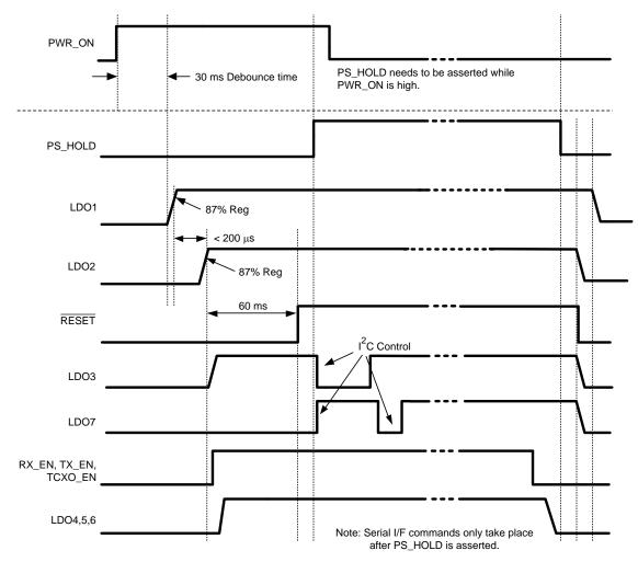
Figure 2. Device Power Up Logic Timing: PWR\_ON
