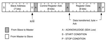
Figure 14. Register Write Format
