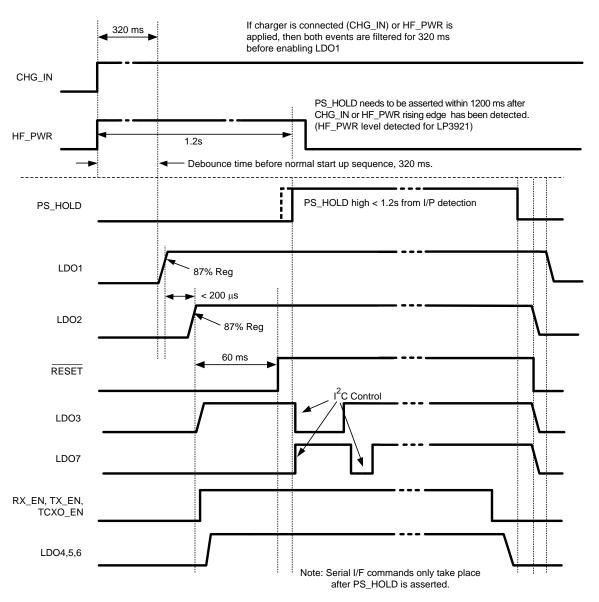
Figure 3. Device Power Up Logic Timing: CHG\_IN, HF\_PWR
