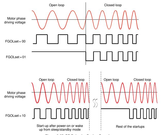
Figure 8-37. FG Behavior During Open Loop
