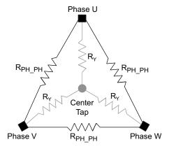
Figure 8-8. Delta-Connected Motor and the Equivalent Wye Connections
