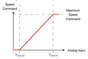
Figure 8-22. Analog-Mode Speed Command
