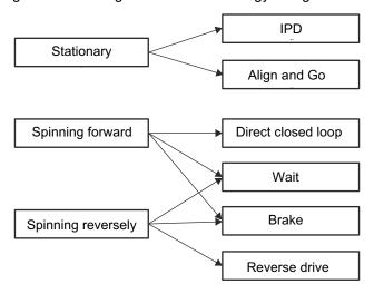
Figure 8-10. Start the Motor Under Different Initial Conditions
