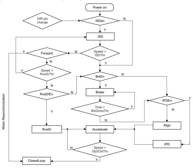
Figure 8-11. Motor Starting-Up Flow
