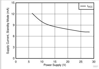
Figure 7-5. Supply Current vs Power Supply Voltage
