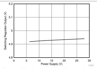
Figure 7-6. Step-Down Regulator Output vs Power Supply Voltage
