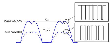
Figure 8-6. Output Voltage Amplitude Adjustment
