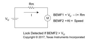
Figure 8-29. Lock Detection 1
