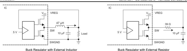
Figure 8-1. Step-Down Regulator Configurations
