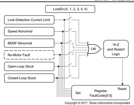
Figure 8-27. Lock Detect and Fault Diagnose
