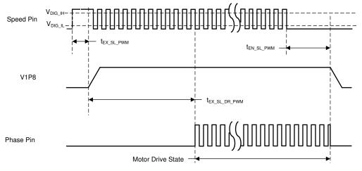
Figure 7-2. DRV10982Q PWM Mode Timing
