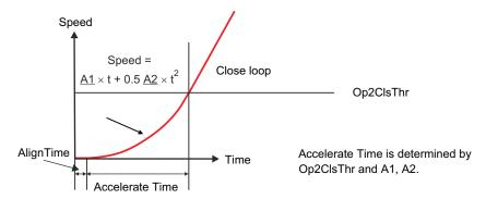
Figure 8-18. Motor Start-Up Process
