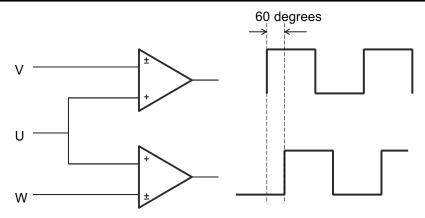
Figure 8-12. Initial Speed Detect Function
