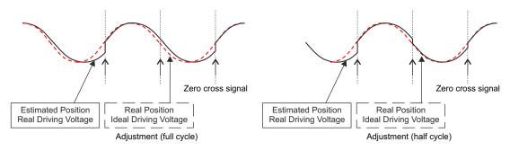
Figure 8-21. Closed-Loop Control Commutation-Adjustment Mode
