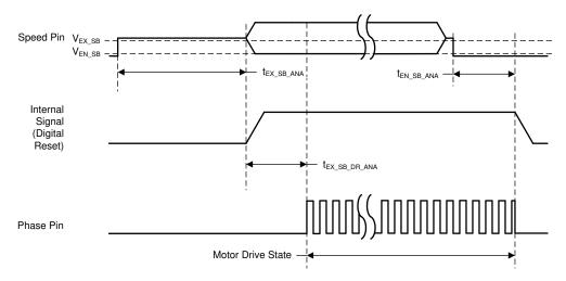
Figure 7-3. DRV10982SQ Analog Mode Timing
