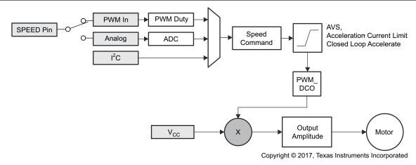
Figure 8-3. Multiplexing the Speed Command to the Output Amplitude Applied to the Motor
