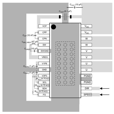
Figure 11-1. Layout Diagram
