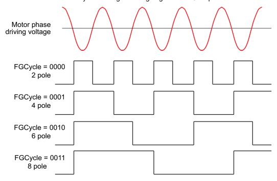
Figure 8-36. FG Frequency Divider
