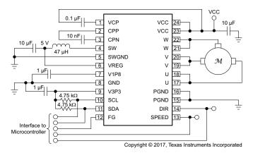
Figure 9-1. Typical Application Schematic
