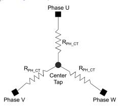
Figure 8-7. Wye-Connected Motor Phase Resistance
