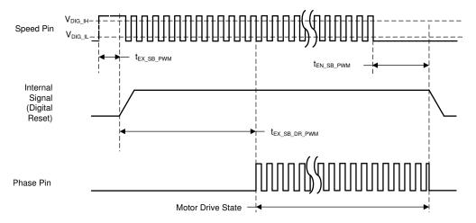
Figure 7-4. DRV10982SQ PWM Mode Timing
