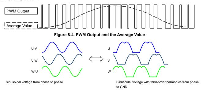
Figure 8-5. Representing Sinusoidal Voltages With Third-Order Harmonic Output
