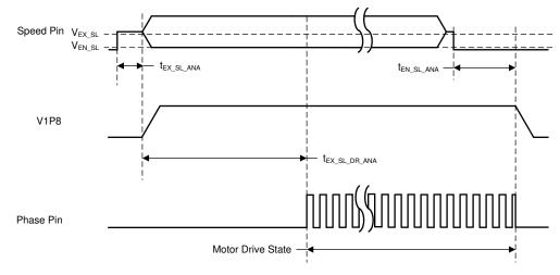
Figure 7-1. DRV10982Q Analog Mode Timing
