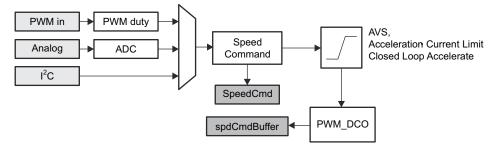
Figure 8-38. SpeedCmd and spdCmdBuffer Registers
