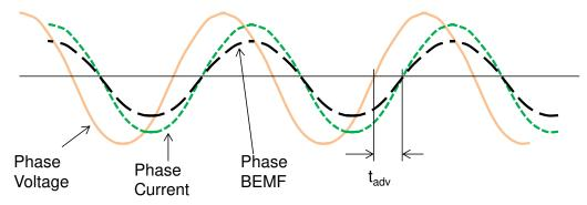
Figure 8-25. Advance Time (t<sub>adv</sub>) Definition
