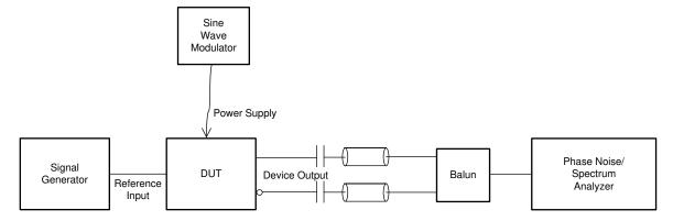
Figure 16. PSNR Test Configuration
