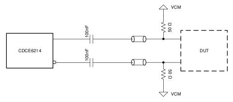
Figure 21. LVDS Output - AC-Coupled
