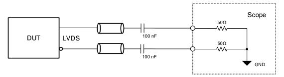
Figure 11. LVDS Output Test Configuration, AC-Coupled
