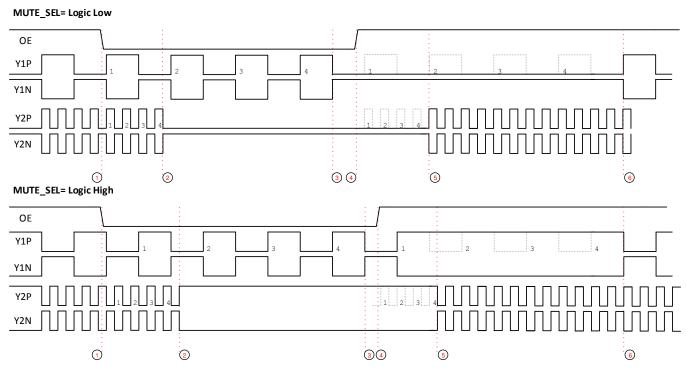
Figure 32. Individual Output Enable and Disable
