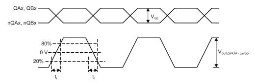
Figure 14. Differential Output Voltage and Rise/Fall Time
