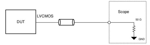
Figure 10. LVCMOS Output Test Configuration
