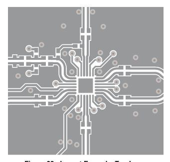
Figure 39. Layout Example, Top Layer
