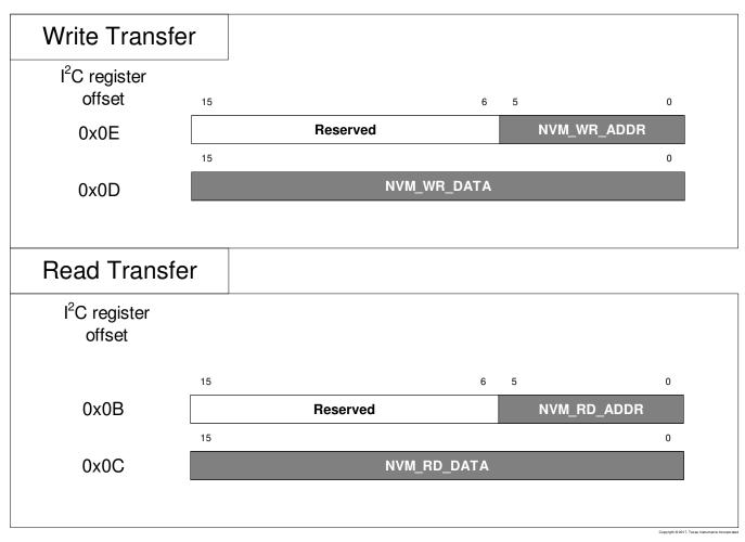
Figure 34. EEPROM Direct Access Using I<sup>2</sup>C
