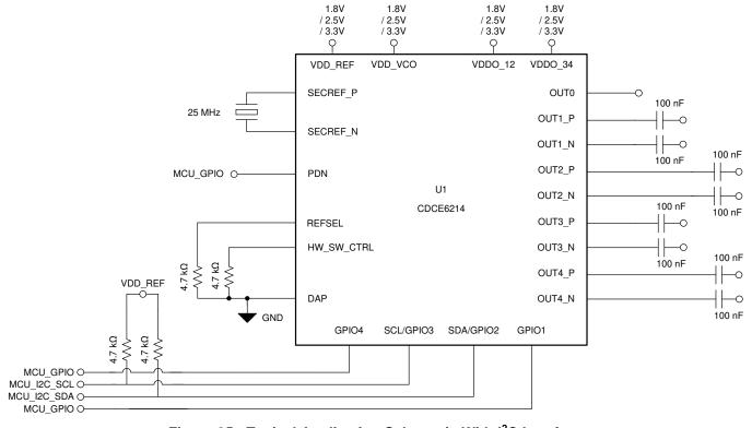
Figure 35. Typical Application Schematic With I<sup>2</sup>C Interface
