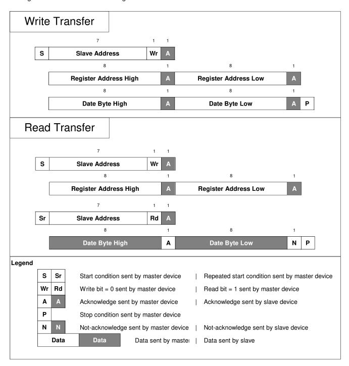
Figure 33. I<sup>2</sup>C-Compatible Serial Interface, Supported Protocol
