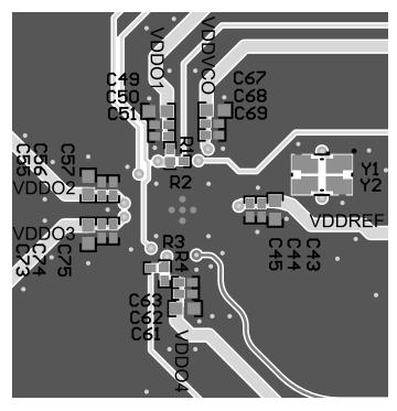
Figure 40. Layout Example, Bottom Layer
