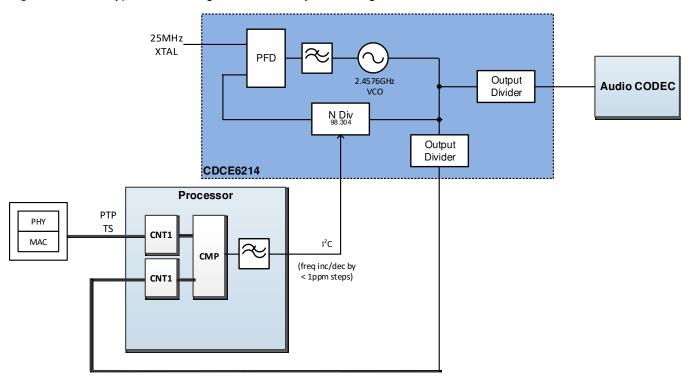
Figure 36. eAVB System Block Diagram Using CDCE6214
