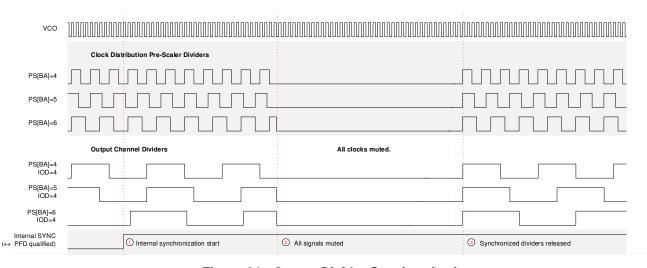
Figure 31. Output Divider Synchronization
