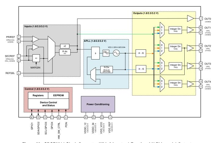
Figure 23. CDCE6214 Clock Generator With 2 Inputs, 1 Fractional-N PLL, and 4 Outputs
