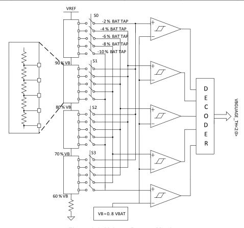
Figure 9-3. Voltage Battery Monitor
