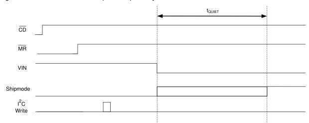
Figure 9-1. CD, MR and VIN Sequencing for Ship Mode Entry Through I<sup>2</sup>C Command
