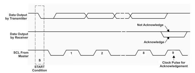
Figure 9-9. Acknowledge on the I<sup>2</sup>C Bus
