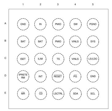
Figure 7-1. YFP Package 25-Pin DSBGA Top View
