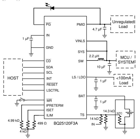
Figure 10-1. Typical Application Circuit
