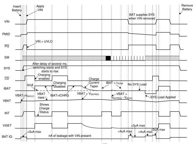
Conditions: PGB\_MRS = 0, TE = 1, SW\_LDO = 1, VINDPM\_ON = 0,  $\overline{PG}$  and INT pulled up to SYS, EN\_INT = 1
