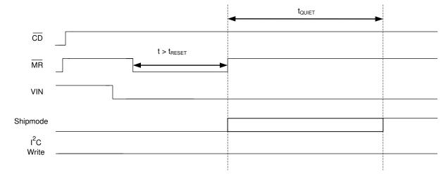
Figure 9-2. CD, MR and VIN Sequencing for Ship Mode Entry Through Long MR Button Press
