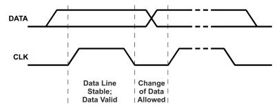
Figure 9-8. Bit Transfer on the Serial Interface
