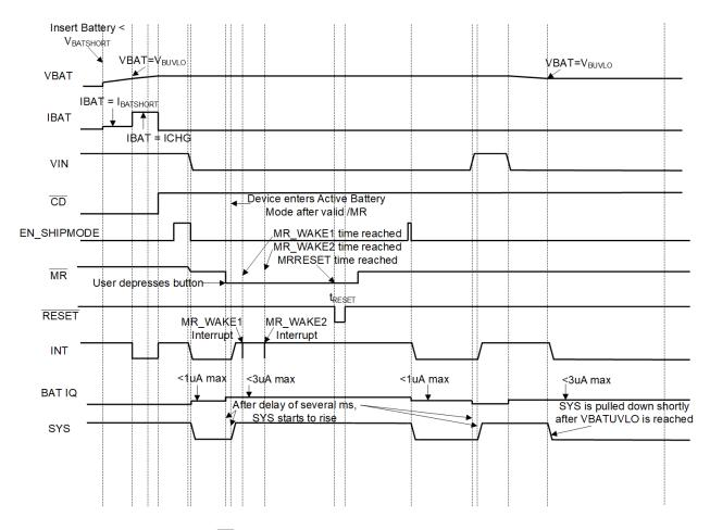
Conditions: SW\_LDO = 1, MRREC = 1,  $\overline{PG}$  and INT pulled up to SYS, ISYS = 10  $\mu$ A, EN\_INT = 1
