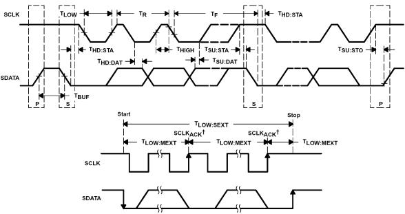
SCLK<sub>ACK</sub> is the acknowledge-related clock pulse generated by the master.
