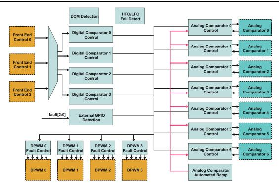
图 9-12. Fault Mux Block Diagram
