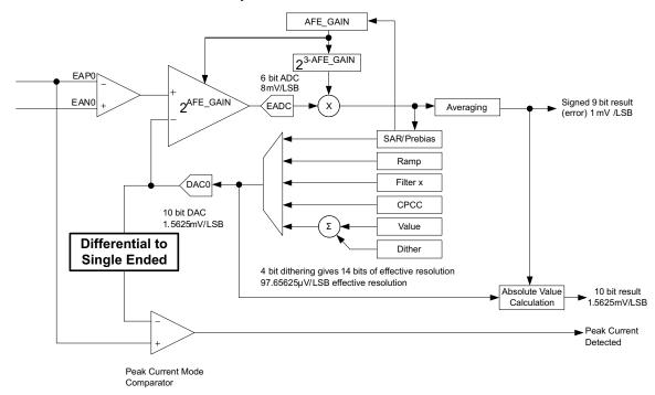
图 10-9. Differential to Single-Ended Comparator Function
