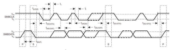
图 8-1. I<sup>2</sup>C/SMBus/PMBus Timing Diagram
