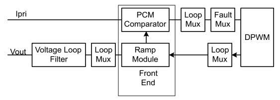
图 10-8. Peak Current Detection Function
