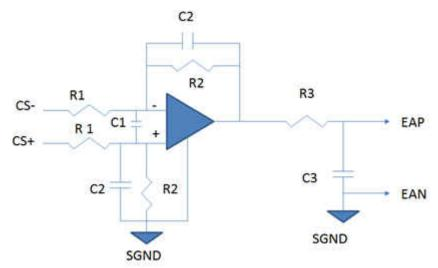
图 12-2. Current Amplifier Connected With EADC
