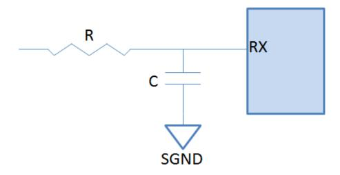
图 12-6. Termination for Communication Port (UART)
