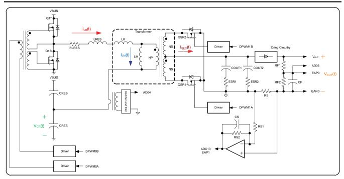
图 9-3. Secondary-Referenced Half-Bridge Resonant LLC Control With Synchronous Rectification
