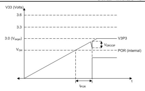
图 11-1. V33 Voltage Dip When POR is Activated
