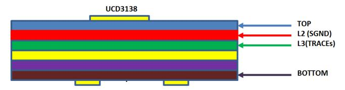
图 12-7. Single Ground Plane for a Power Module Design
