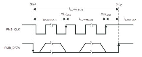
图 8-2. Bus Timing in Extended Mode
