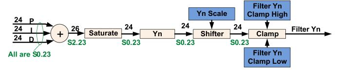
图 9-7. Output Section of the Filter
