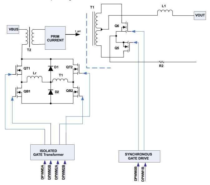
图 10-2. Schematic - PSFB Power Stage
