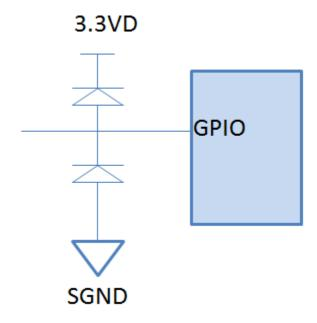
图 12-3. Clamping Diodes for GPIO
