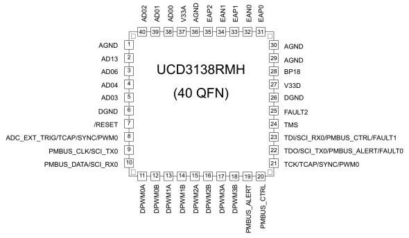
NOTE: The RMH package is not recommended for new designs. It has thinner package height compared to the RHA package. There are also four corner pins on the RMH package. The corner anchor pins and thermal pad should be soldered for robust mechanical performance and should be tied to the appropriate ground signal.
