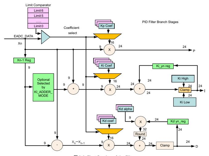
图 9-6. First Section of the Filter
