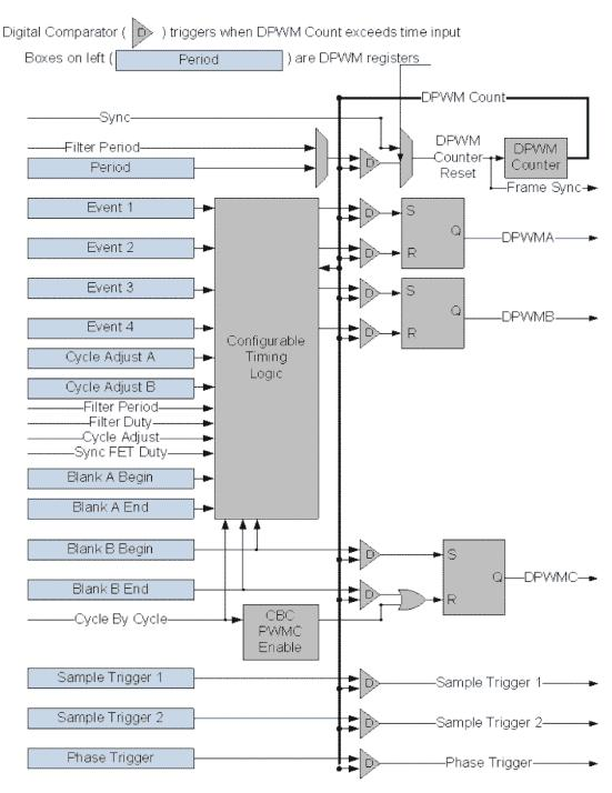
图 10-4. Fixed Signals to Bridge
