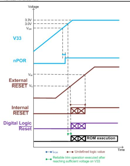
图 11-2. Recommended Timing Diagram of V33 and RESET for UCD3138 and UCD3138064
