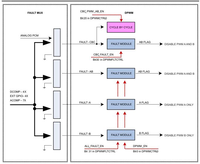
The Fault Mux Module provides a multitude of fault protection functions within the UCD3138 high-speed loop (front end control, filter, DPWM and loop Mux modules). The Fault Mux Module allows highly configurable fault generation based on digital comparators, high-speed analog comparators and external fault pins. Each of the fault inputs to the DPWM modules can be configured to one or any combination of the fault events provided in the Fault Mux Module.
