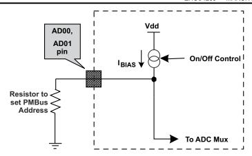
图 9-13. PMBus Address Detection Method
