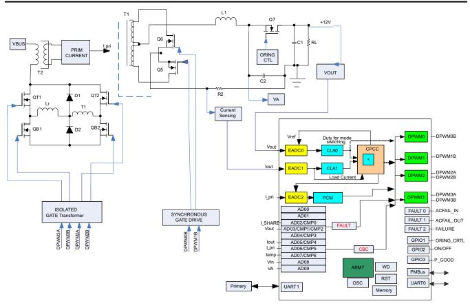
图 9-2. Secondary-Referenced Phase-Shifted Full Bridge Control With Synchronous Rectification
