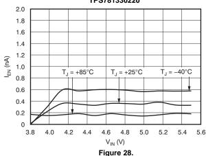
ENABLE PIN HYSTERESIS vs TEMPERATURE I<sub>OUT</sub> = 1mA, TPS781330220
