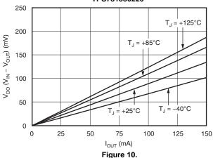
DROPOUT VOLTAGE vs TEMPERATURE  $V_{VSET}$  = 0.4V,  $V_{OUT}$  = 3.3V (typ),  $V_{IN}$  = 0.95 ×  $V_{OUT}$  (typ) TPS781330220
