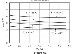
GROUND PIN CURRENT vs INPUT VOLTAGE  $I_{OUT}$  = 50mA,  $V_{VSET}$  = 0.4V,  $V_{OUT}$  = 3.3V TPS781330220
