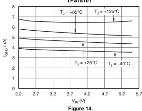
GROUND PIN CURRENT vs INPUT VOLTAGE  $I_{OUT}$  = 150mA,  $V_{VSET}$  = 1.2V,  $V_{OUT}$  = 2.2V TPS781330220
