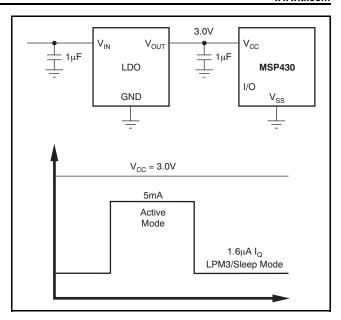
Figure 50. Typical LDO without DVS
