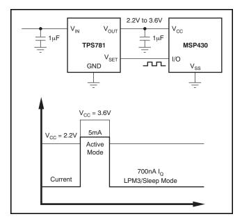
Figure 51. TPS781 with Integrated DVS
