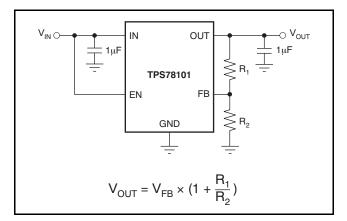
Figure 49. TPS78101 Adjustable LDO Regulator Programming
