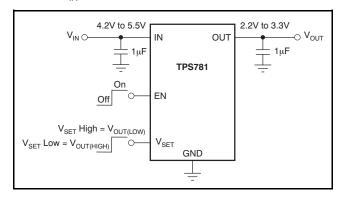
Figure 48. Typical Application Circuit
