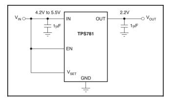
Figure 53. Circuit to Tie Both EN and V<sub>SET</sub> High
