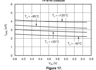
GROUND PIN CURRENT vs INPUT VOLTAGE  $I_{OUT}$  = 150mA,  $V_{OUT}$  = 1.22V TPS78101
