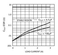
Figure 33. Minimum ESR vs Output Load Current
