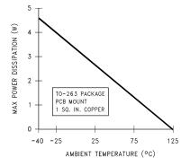
Figure 35. Maximum power dissipation vs ambient temperature for DDPAK/TO-263 package
