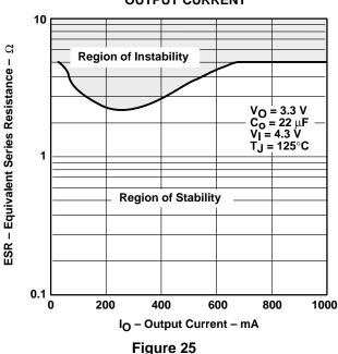
$<sup>\</sup>dagger$  Equivalent series resistance (ESR) refers to the total series resistance, including the ESR of the capacitor, any series resistance added externally, and PWB trace resistance to  $C_0$ .
