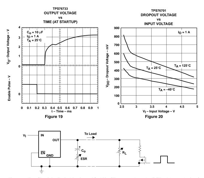
Figure 21. Test Circuit for Typical Regions of Stability (Figures 22 through 25) (Fixed Output Options)
