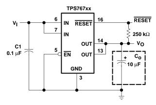
Figure 26. Typical Application Circuit (Fixed Versions)
