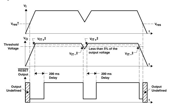
$<sup>^\</sup>dagger$  V<sub>res</sub> is the minimum input voltage for a valid  $\overline{\text{RESET}}$ . The symbol V<sub>res</sub> is not currently listed within EIA or JEDEC standards for semiconductor symbology.
