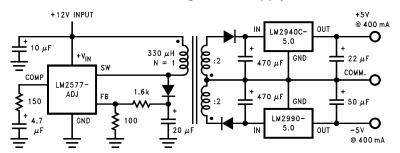
Figure 20. Post Regulator for an Isolated Switching Power Supply
