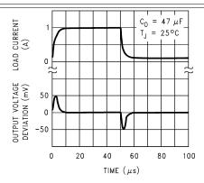
Figure 7. LM2990-5 and LM2990-5.2 Line Transient Response
