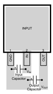
Figure 26. LM2990 TO-263 Board Layout
