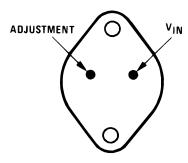
Figure 6-1. LM117K K Package 2-Pin TO-3 (Metal Can) Bottom View
