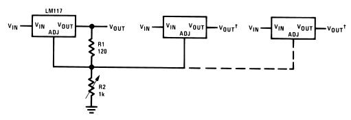
\*All outputs within ±100 mV †Minimum load = 10 mA
