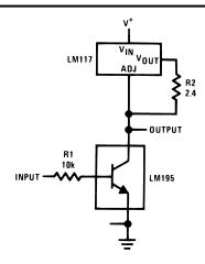
Figure 9-11. High Gain Amplifier
