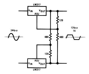
Figure 9-18. AC Voltage Regulator
