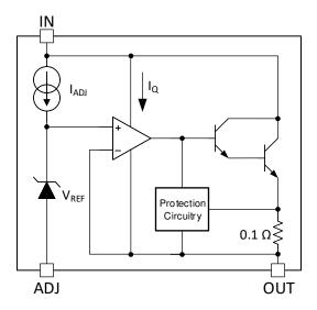
Figure 8-1. Functional Block Diagram
