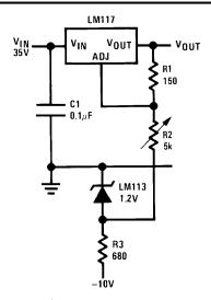
Full output current not available at high input-output voltages
