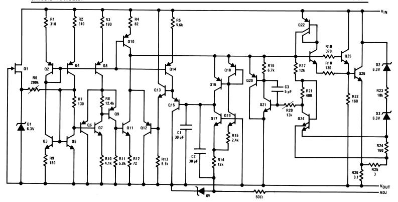
Figure 8-2. Simplified Device Schematic
