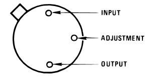
Figure 6-2. LM117H, LM117NDT NDT Package 3-Pin TO-39 (Metal Can) Bottom View
