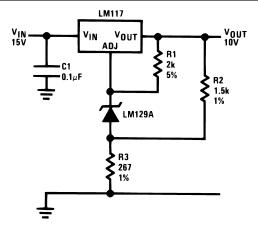
Figure 9-4. High Stability 10-V Regulator
