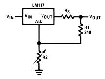
Figure 8-3. Regulator With Line Resistance in Output Lead
