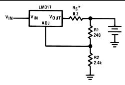
\*R<sub>S</sub>—sets output impedance of charger: Z<sub>OUT</sub> = R<sub>S</sub>
