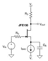
图 9-4. Common-Source Amplifier With Current-Source Biasing
