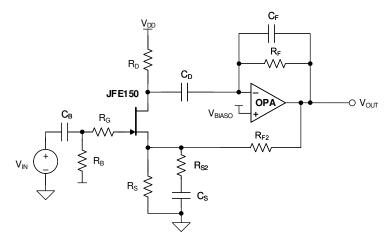
图 9-5. Low Noise, High Input Impedance Composite Amplifier
