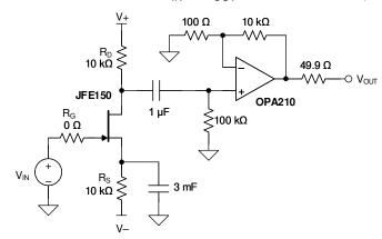
图 7-1. AC Measurement Reference Schematic
