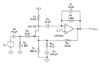
图 9-6. Low-Noise, High-Input-Impedance Composite Amplifier
