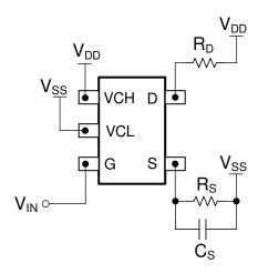
图 11-1. JFE150 Layout Example, Common Source Configuration
