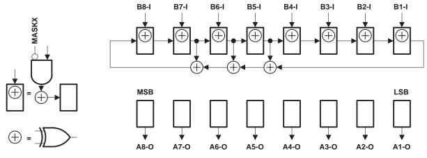
Figure 11. 8-Bit PSA/COUNT Configuration (OEA = 1, OEB = 0)
