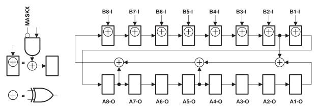
Figure 7. 16-Bit PSA Configuration (OEA = 1, OEB = 0)
