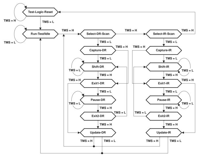
Figure 1. TAP-Controller State Diagram
