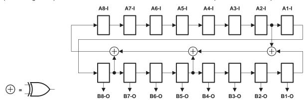
Figure 4. 16-Bit PRPG Configuration (OEA = 0, OEB = 1)
