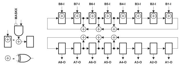
Figure 9. 8-Bit PSA/PRPG Configuration (OEA = 1, OEB = 0)
