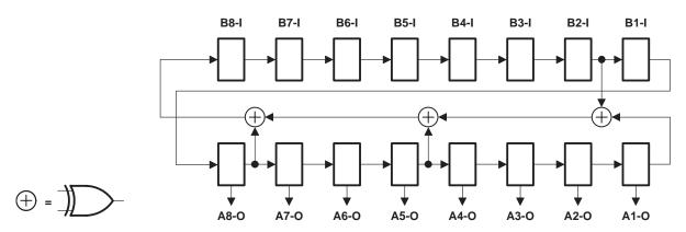
Figure 5. 16-Bit PRPG Configuration (OEA=1, OEB=0)
