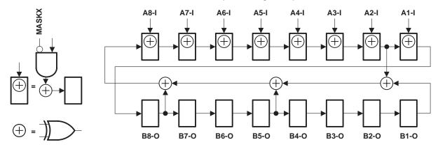
Figure 6. 16-Bit PSA Configuration (OEA = 0, OEB = 1)
