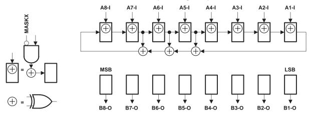
Figure 10. 8-Bit PSA/COUNT Configuration (OEA = 0, OEB = 1)
