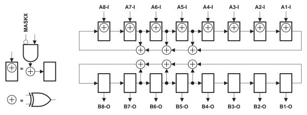
Figure 8. 8-Bit PSA/PRPG Configuration (OEA = 0, OEB = 1)
