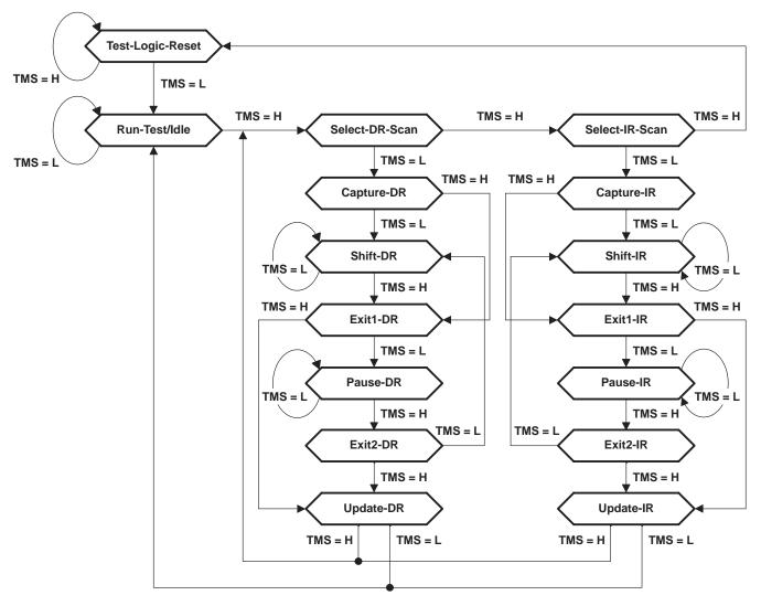
Figure 1. TAP-Controller State Diagram
