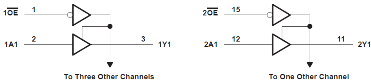
图 8-1. Logic Diagram (Positive Logic)
