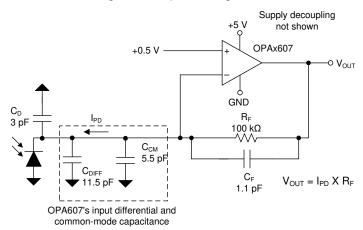
图 9-1. Wideband, High-Sensitivity, Transimpedance Amplifier
