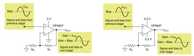
图 8-6. Single-Supply and Dual-Supply Operation
