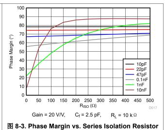
a o-z. Phase margin vs. Series isolation Resistor
