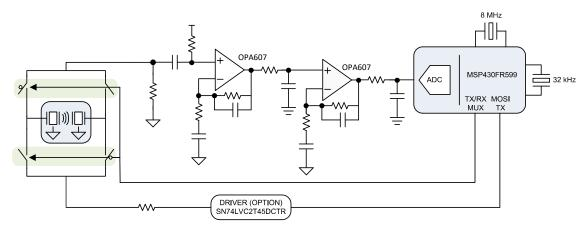
图 9-15. High-Gain Ultrasonic Front-End
