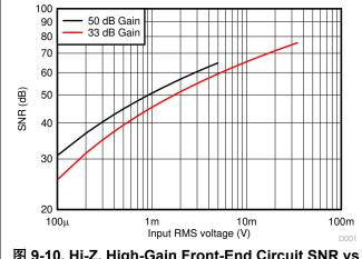
图 9-10. Hi-Z, High-Gain Front-End Circuit SNR vs Input
