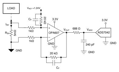
图 9-12. Low Side Current Sensing
