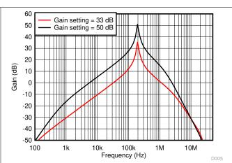
图 9-11. Hi-Z, High-Gain Front-End Circuit Gain vs Frequency
