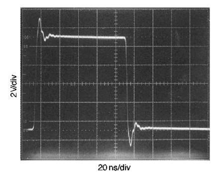
Figure 49. Improperly Terminated Signal
