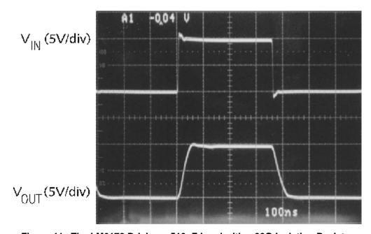
Figure 44. The LM6172 Driving a 510pF Load with a  $30\Omega$  Isolation Resistor
