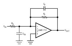
Figure 46. Compensating for Input Capacitance
